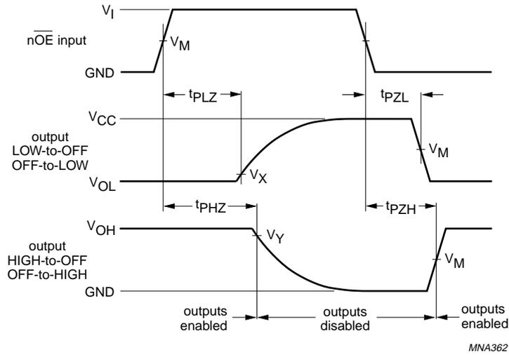
For 74HC2G125:  $V_M = 50\%$ ;  $V_1 = \text{GND to } V_{CC}$ .
