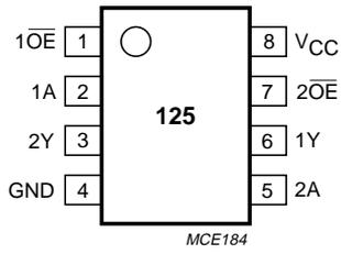
Fig.1 Pin configuration.
