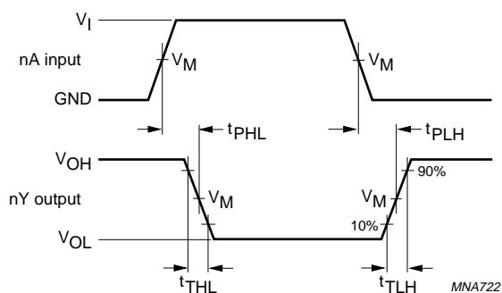
For HC3G:  $V_M = 50\%$ ;  $V_I = \text{GND to } V_{cc}$ .For HCT3G:  $V_M = 1.3 \text{ V}$ ;  $V_I = \text{GND to } 3.0 \text{ V}$ .
