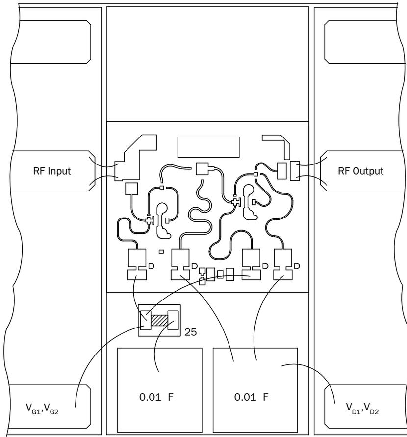
RF connections: bond using two 1-mil diameter, 20 to 25 - mil-length gold bond wires at both RF Input and RF Output for optimum RF performance.
