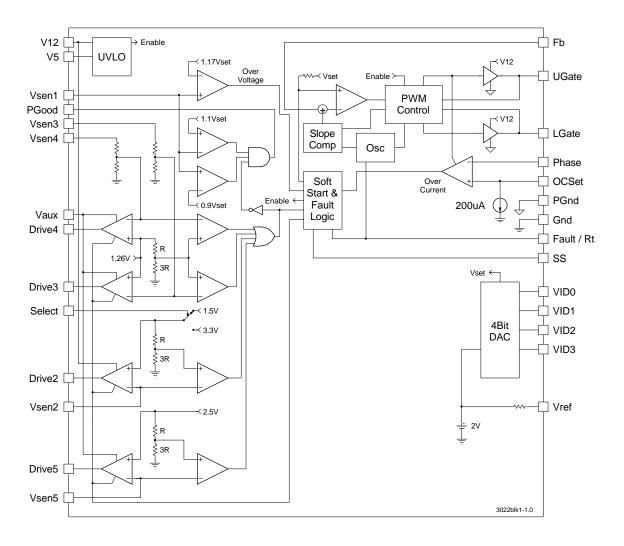
Figure 1 - Simplified block diagram of the US3022.
