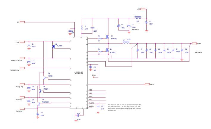
Figure 2 - Typical application of US3022 for an on board DC-DC converter providing power for the Vcore, GTL+, 1.8V chip set supply, 2.5V clock supply as well as auto select AGP supply for the next generation PC applications.
