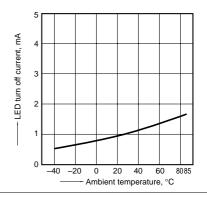
9. Off state leakage current
