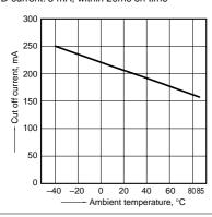
5. LED operate current vs. ambient temperature characteristics
