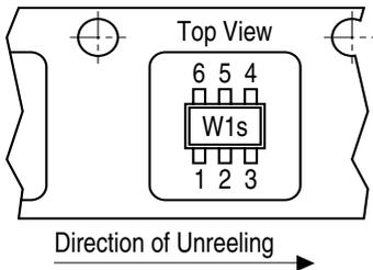
Marking on SOT-363 package (for example W1s) corresponds to pin 1 of device
