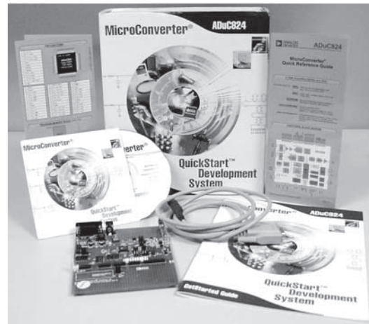
Figure 65. Components of the QuickStart Development System
