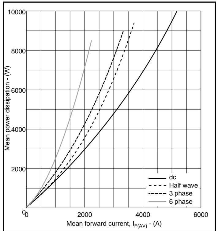
**Fig.3 Dissipation curves**
