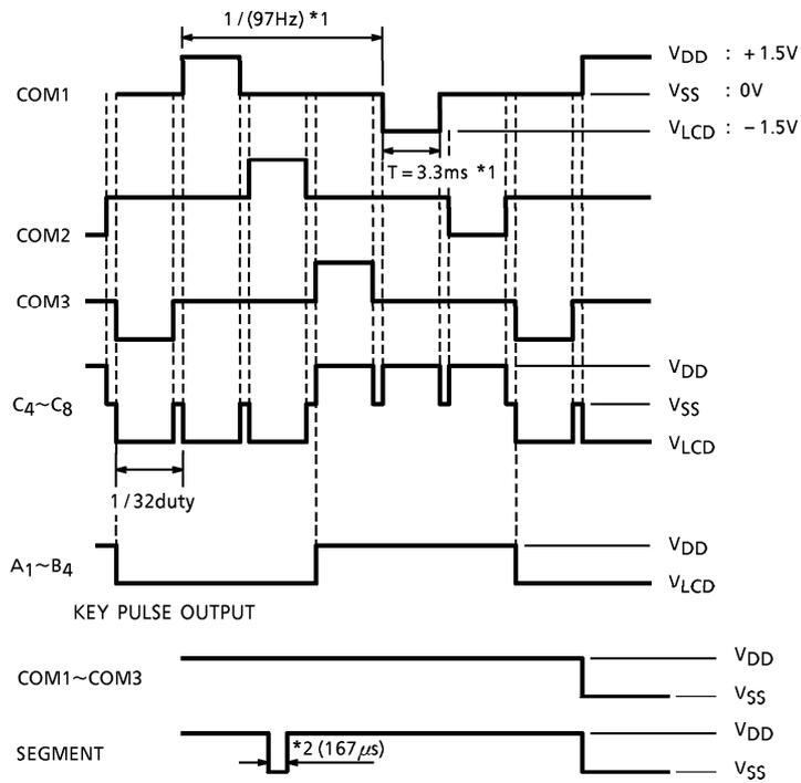
(\*1)  $f_{\phi} = 7\text{kHz}$
