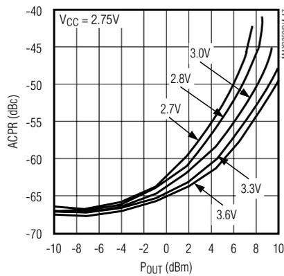
**CASCADE ACPR vs. P<sub>OUT</sub> AND V<sub>BAT</sub>**
