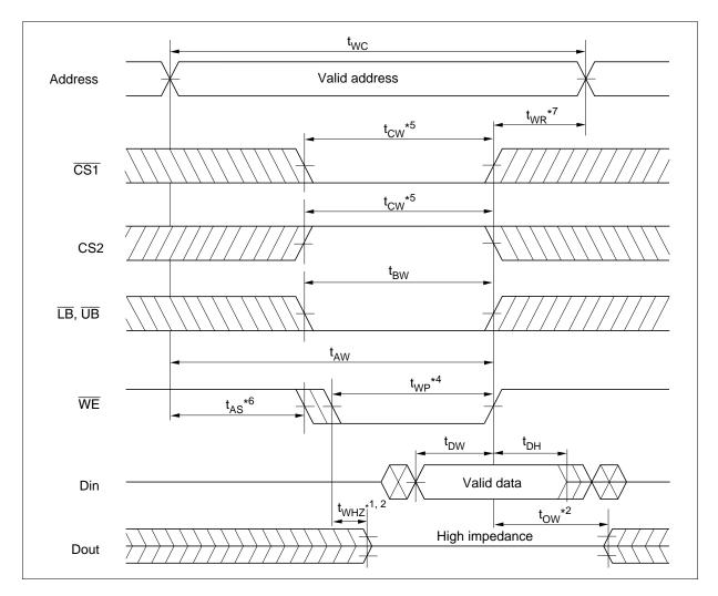
Write Cycle (2) ( $\overline{CS}$  Clock,  $\overline{OE} = V_{IH}$ )
