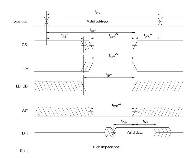
Write Cycle (3) ( $\overline{LB}$ ,  $\overline{UB}$  Clock,  $\overline{OE} = V_{IH}$ )
