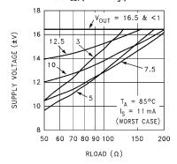
The curves do not include heat removal or forcing air, or the simple fact that the package will probably be attached to a circuit board, which can also provide some form of heat removal. Larger temperature and voltage ranges are possible with heat removal and forcing air past the part.
