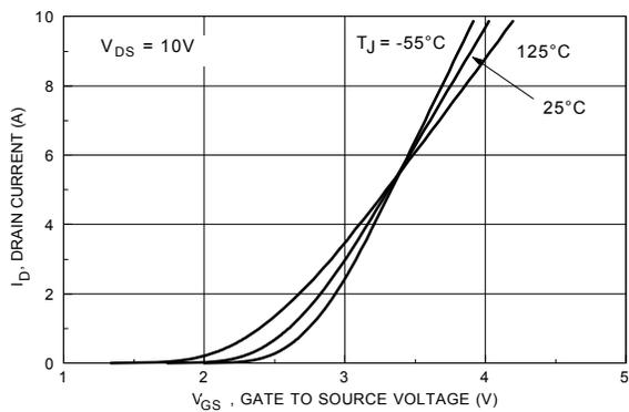
Figure 5. Transfer Characteristics.
