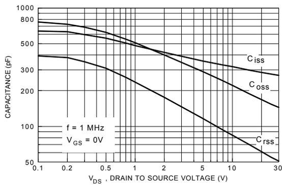
**Figure 9. Capacitance Characteristics.**
