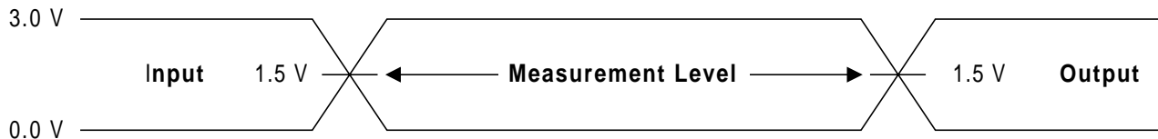
Figure 16. Input Waveforms and Measurement Levels
