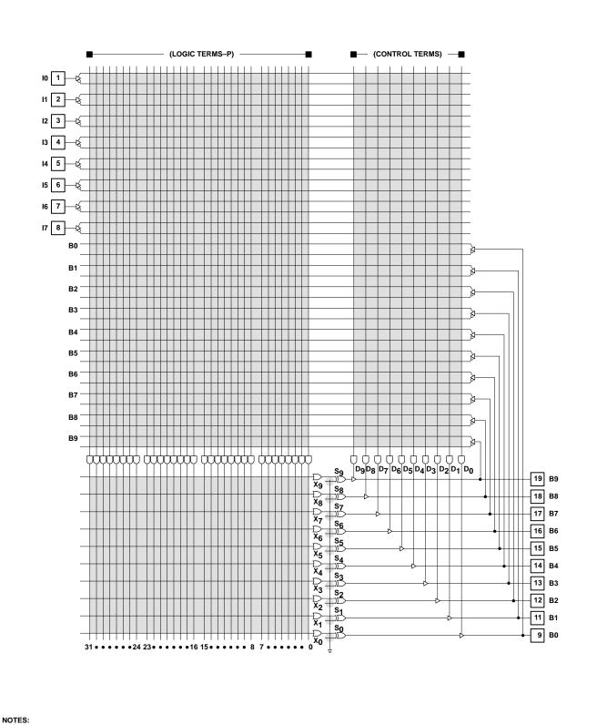
All programmed 'AND' gate locations are pulled to logic "1".
