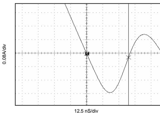
**Figure 13. Non-SyncFET (FDS7066N3) body diode reverse recovery characteristic.**
