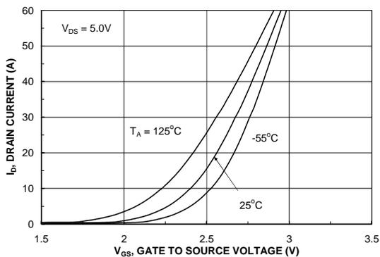
Figure 5. Transfer Characteristics.
