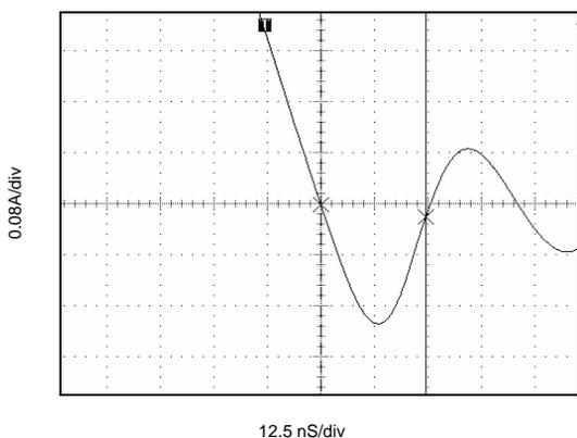
**Figure 12. FDS7066ASN3 SyncFET body diode reverse recovery characteristic.**
