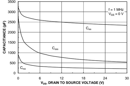
**Figure 8. Capacitance Characteristics.**
