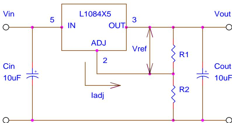
$$V_o = V_{ref} (1+R_2/R_1) + I_{adj} \times R_2$$
