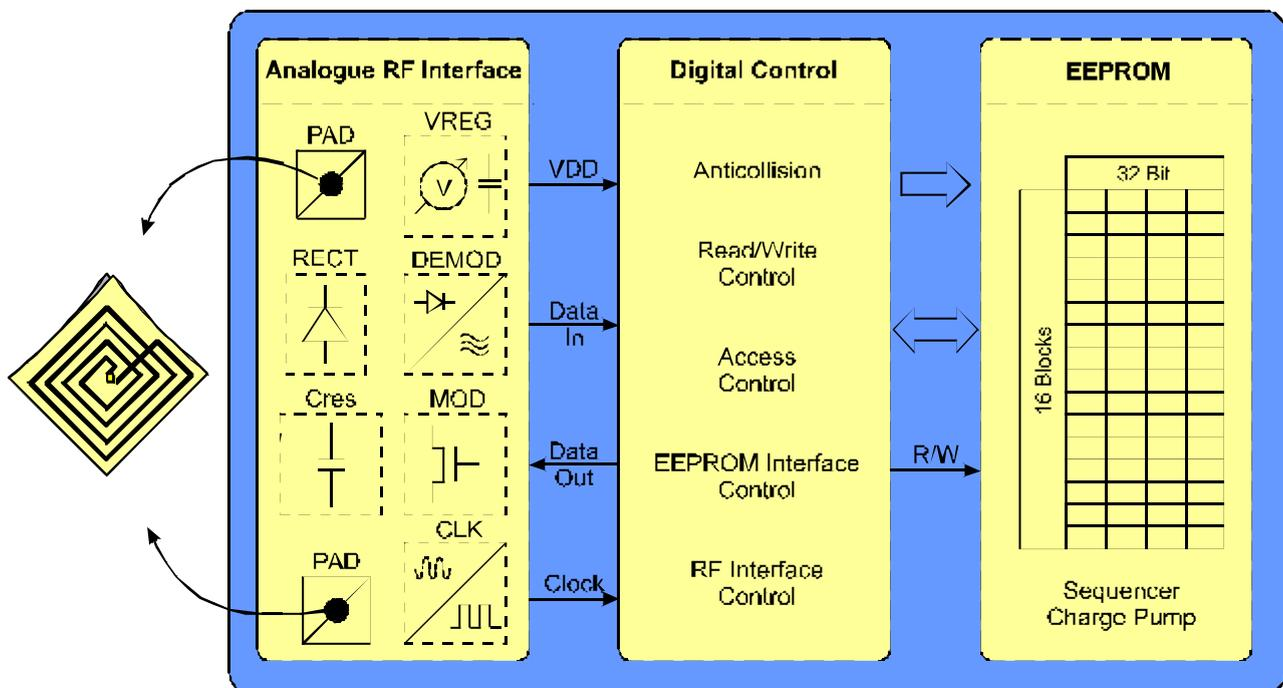
The label requires no internal power supply. Its contactless interface generates the power supply and the system clock via the resonant circuitry by inductive coupling to the reader. The interface also demodulates data that are transmitted from the reader to the I•CODE Label, and modulates the electromagnetic field for data transmission from the I•CODE Label to the reader.
