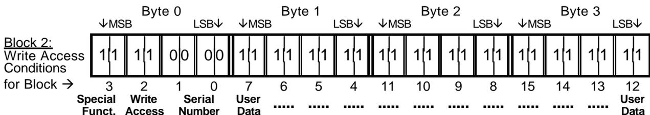
The ones in the 16 pairs of bits have to be cleared together if the corresponding block is wanted to be write protected forever (1|1 → write access enabled, 0|0 → write access disabled). Writing of bit pairs 1|0 or 0|1 to block 2 is not allowed!
