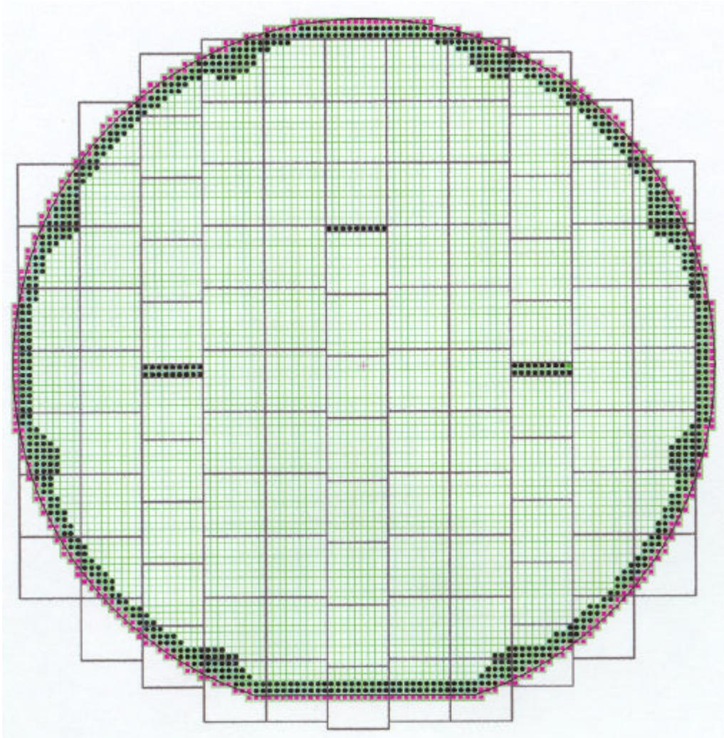
The three black lines show the position of the PCM structures on the 6 inch wafer!
