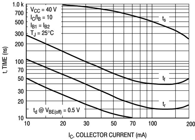
Figure 4. Switching Times
