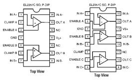
125 MHz Single Supply, Clamping Op Amps
