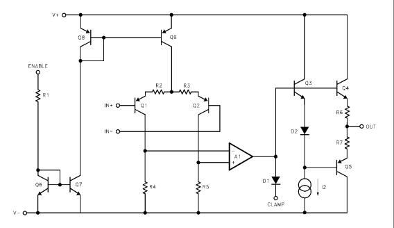
125 MHz Single Supply, Clamping Op Amps
