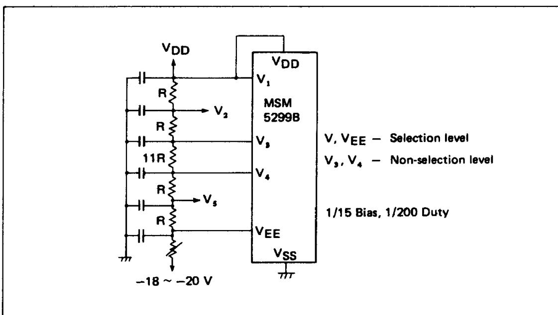
The figure below shows the case when the bias voltage is supplied by using Ope-Amps, which enables the bias source low impedance and low power consumption.
