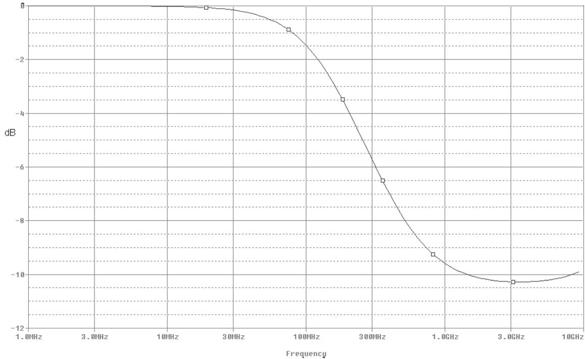
Figure 1. Typical EMI Filter Performance (Simulated)
