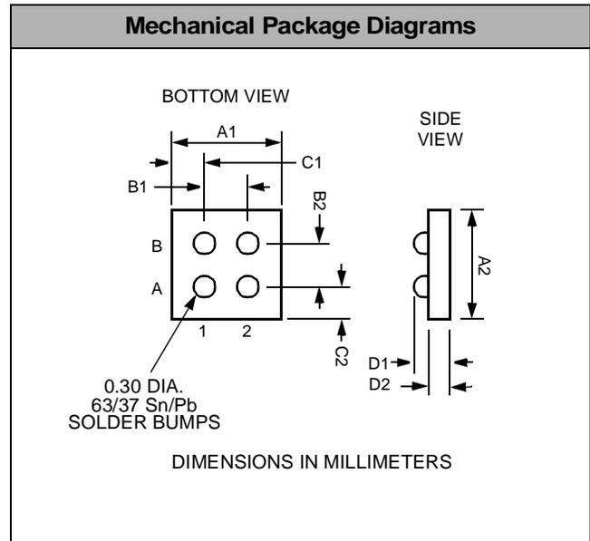
Package Dimensions for CSPE SD301/302/303 Chip Scale Package
