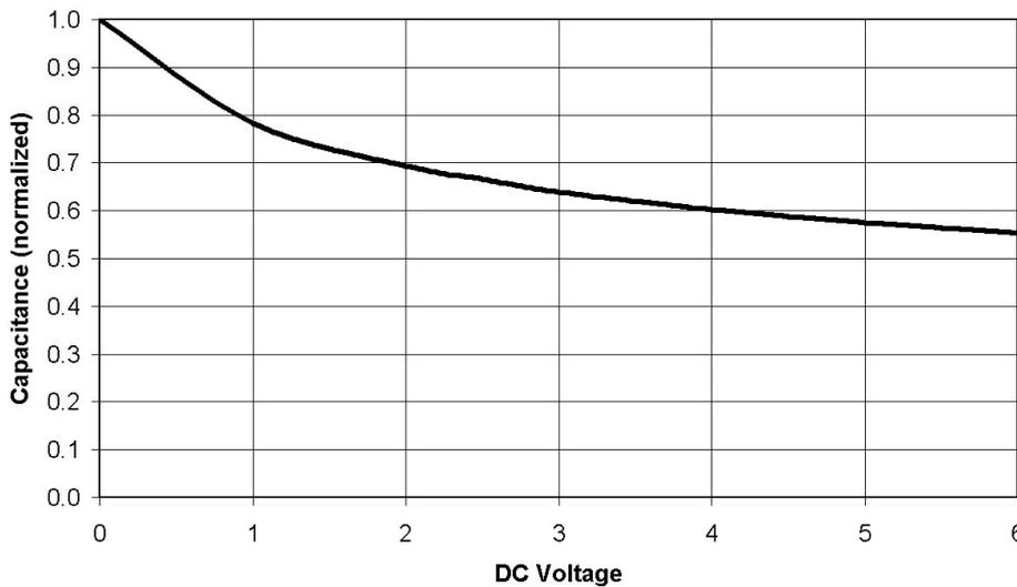
Figure 2. Typical Diode Capacitance VS. Input Voltage (normalized to 0Vdc)
