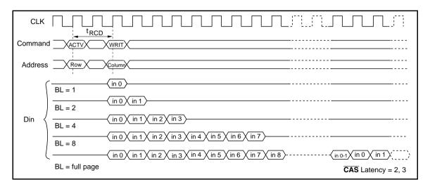
**2. Single write:** A single write operation is enabled by setting OPCODE (A9, A8) to (1, 0). In a single write operation, data is only written to the column address (AY0 to AY7; HM52Y64165F, AY0 to AY8; HM52Y64805F, AY0 to AY9; HM52Y64405F) and the bank select address (A12/A13) specified by the write command set cycle without regard to the burst length setting. (The latency of data input is 0 clock).
