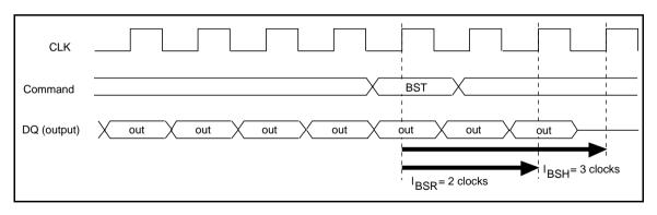
**Burst stop command at burst write:** The burst stop command (BST command) is used to stop data input during a full-page burst write. No data is written in the same clock as the BST command, and in subsequent clocks. In addition, the BST command is only valid during full-page burst mode, and is illegal with burst lengths of 1, 2, 4 and 8. And an interval of t<sub>DPL</sub> is required between last data-in and the next precharge command
