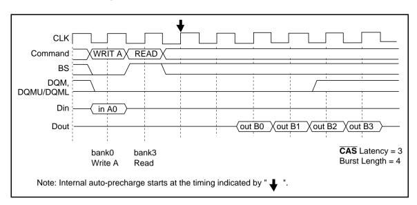
**Same bank:** The consecutive read command from write with auto precharge (the same bank) is illegal. . It is necessary to separate the two commands with a bank active command.
