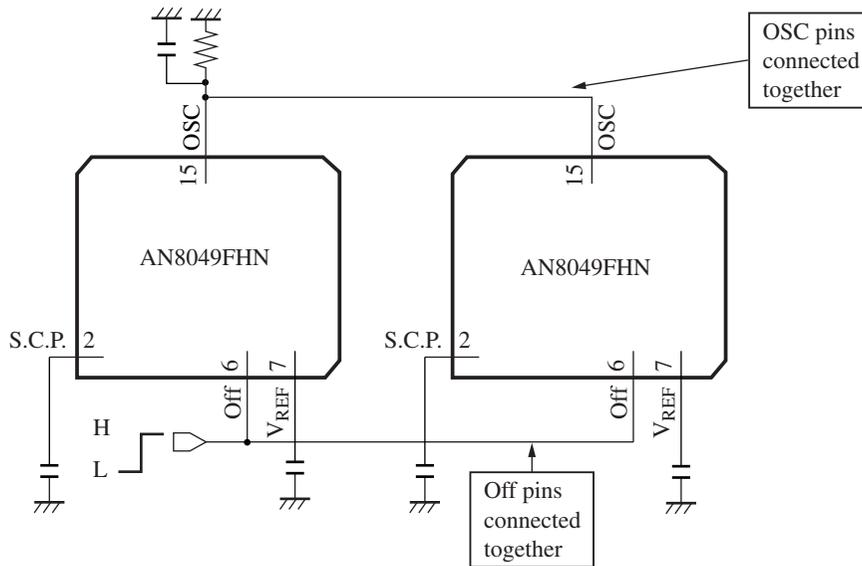
Figure 7. Slave operation circuit example
