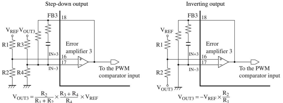
Figure 4. Connection method of error amplifier 3
