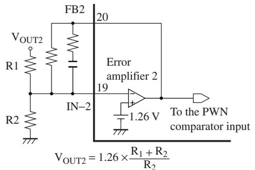
Figure 3. Connection method of error amplifier 2 (Step-up output)
