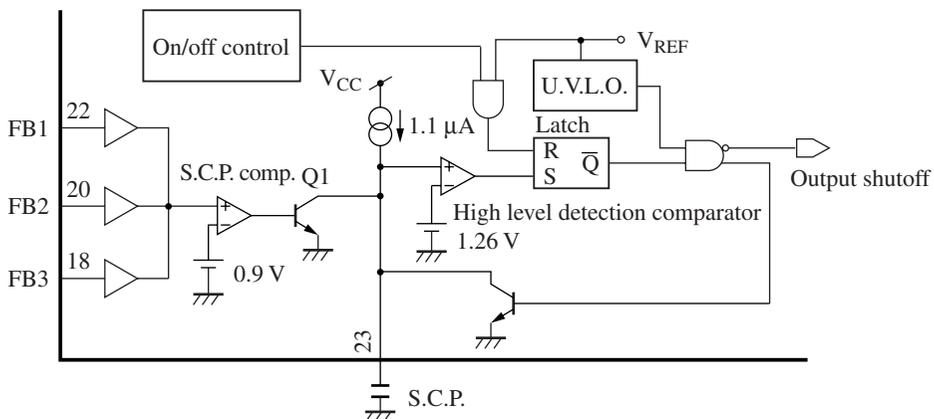
Figure 6. Short-circuit protection circuit
