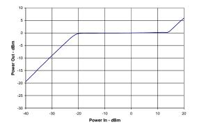
Figure 13 Output Power versus Input Power in AGC Mode at 140MHz.
