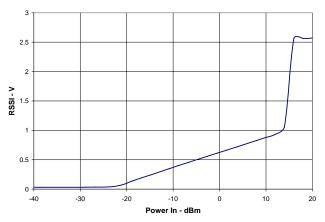
Figure 14. Monitoring the GAIN/DETO RSSI Voltage versus Input Power.
