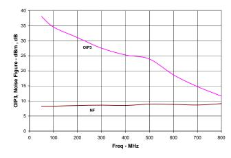
Figure 7.OIP3 and NF vs. Frequency
