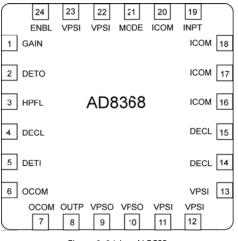
Figure 2. 24-Lead LFCSP
