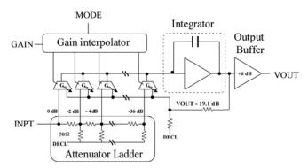
Figure 8. Simplified Block Diagram
