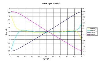
*Figure 10 The gain function can be either an increasing or decreasing function of VGAIN, depending on the MODE pin.*
