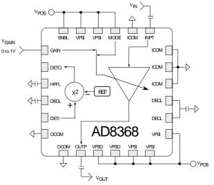
Figure 11. Typical Connections for VGA Mode
