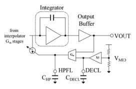
Figure 9. Output Centering Control Loop
