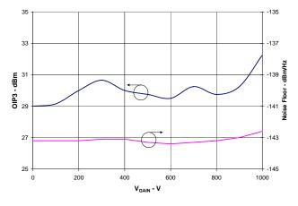
Figure 5. OIP3 and Output Noise Floor vs. V<sub>GAIN</sub> at 140MHz
