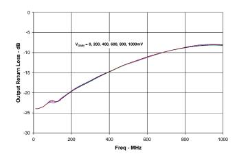
Figure 7. Output Return Loss vs. Frequency
