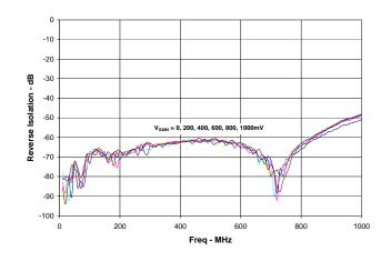
Figure 6. Reverse Isolation vs. Frequency
