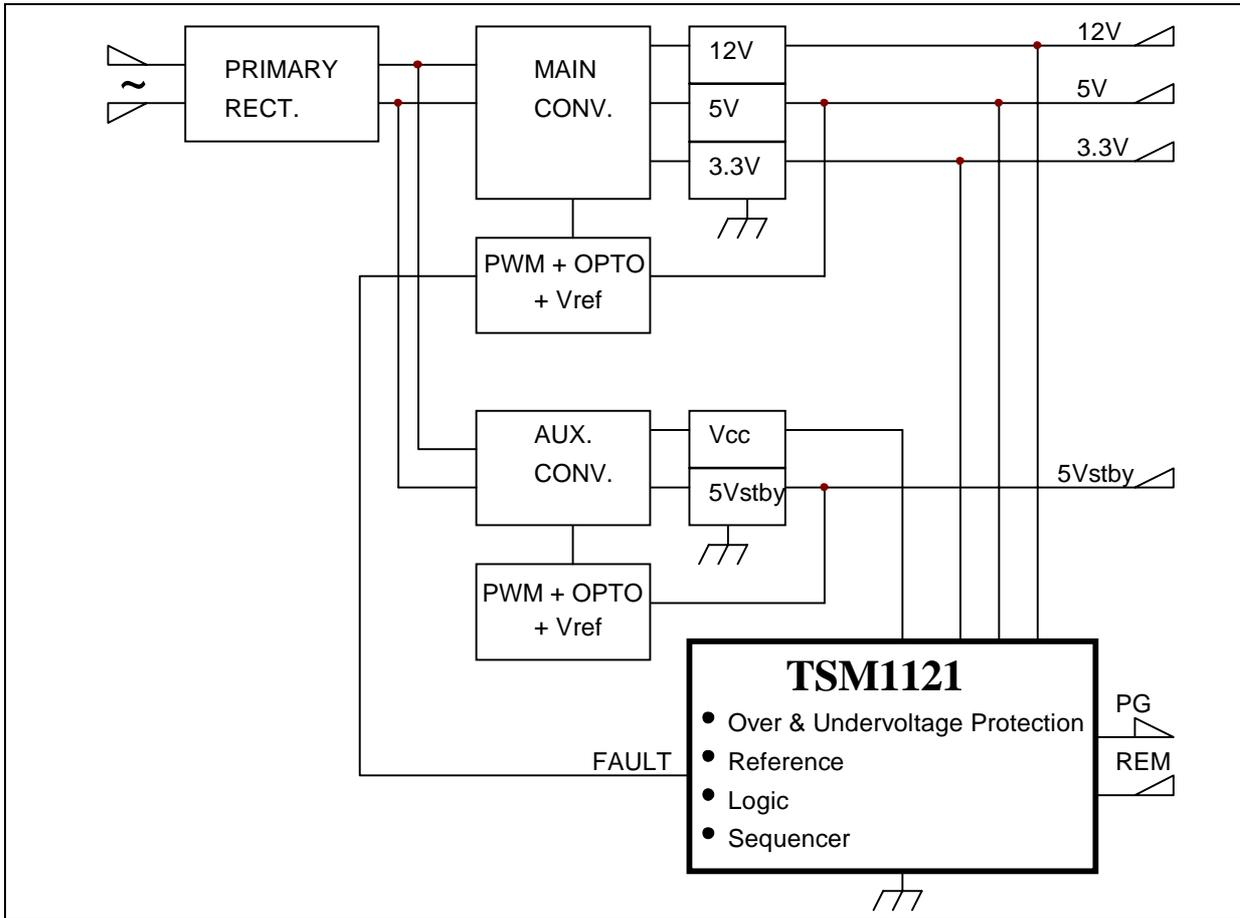
Fig. 2: Internal Schematic
