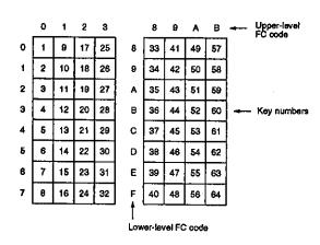
Note that when the appropriate mask option is selected, function codes 97H, A7H, B7H, C7H, D7H, E7H and F7H can also be generated by holding down key 8 and one of keys 16, 24, 32, 40, 48, 56 and 64.
