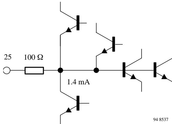
Figure 21. AF output AM sound (Pin 25)
