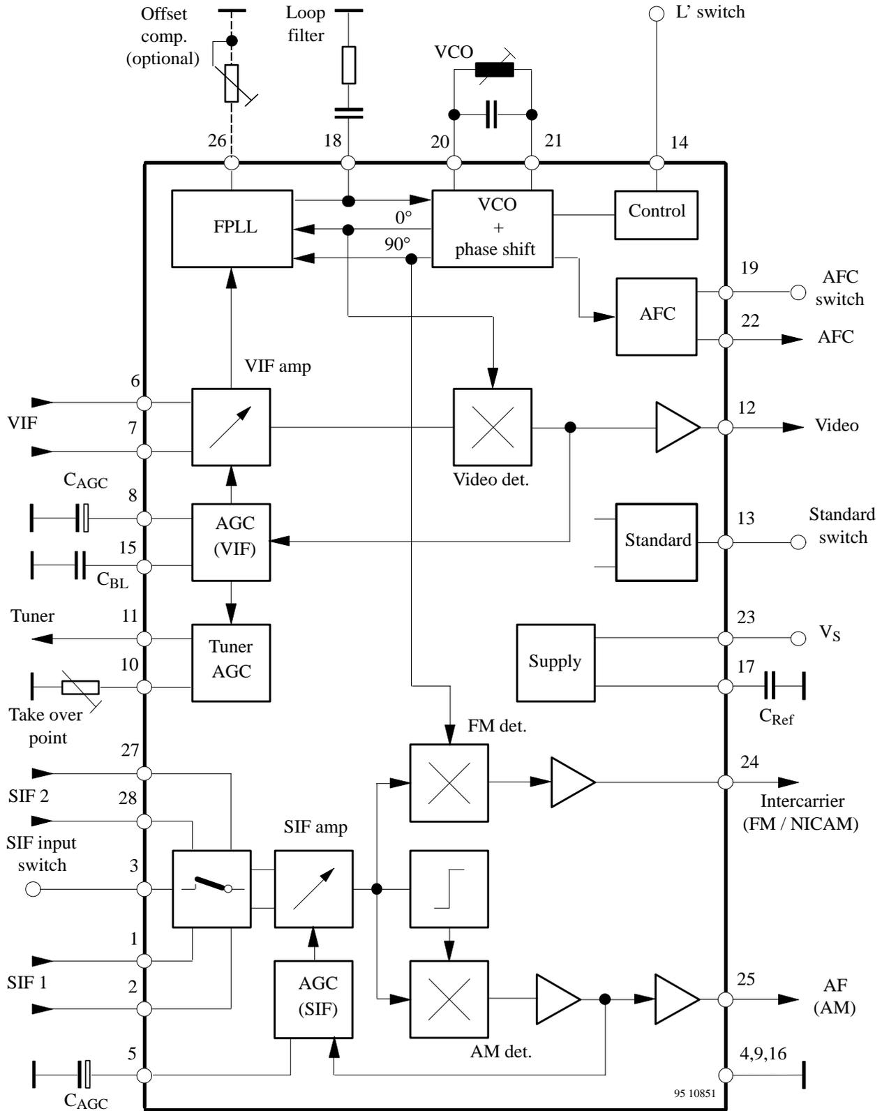
Figure 1. Block diagram
