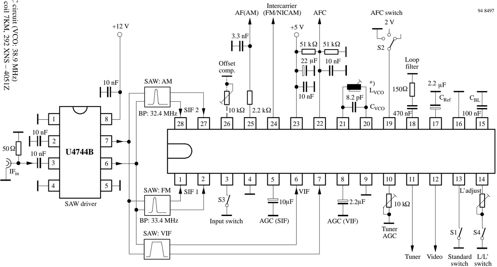
\*) External L/C circuit (VCO: 38.9 MHz) with TOKO coil 7KM, 292 XNS - 4051Z
