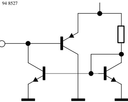
Figure 11. Tuner AGC – output (Pin 11)
