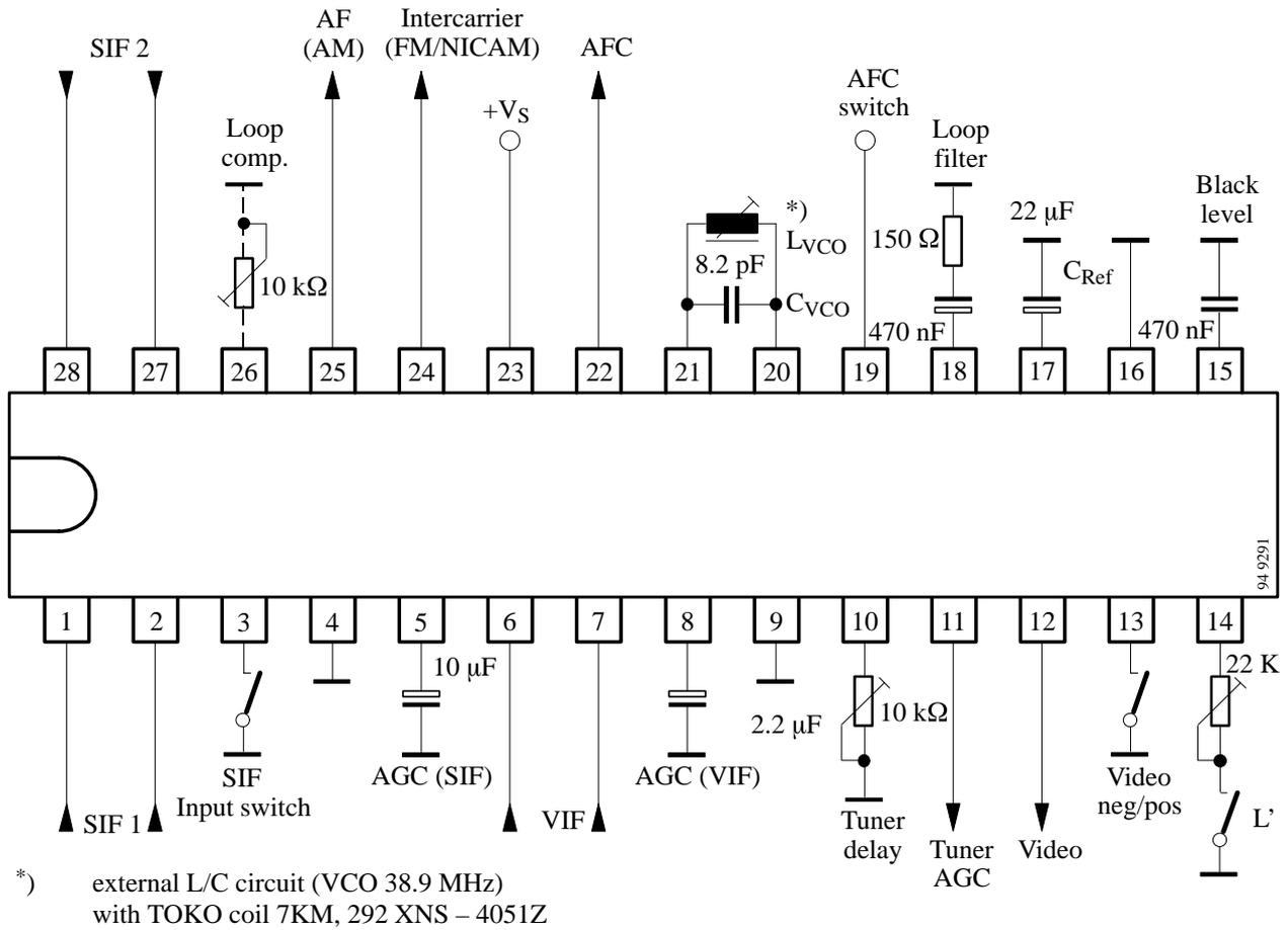
Figure 3. Test circuit
