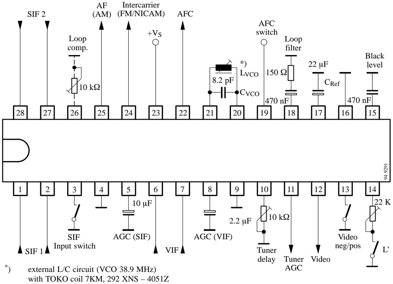
Figure 3. Test circuit
