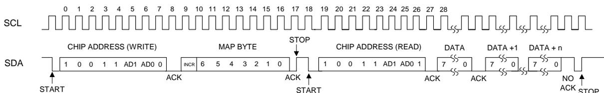
**Figure 23. Control Port Timing, I<sup>2</sup>C Read**
