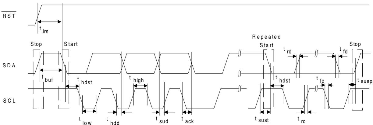
**Figure 3. Control Port Timing - I<sup>2</sup>C Format**
