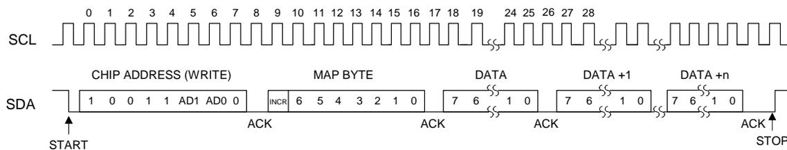
**Figure 22. Control Port Timing, I<sup>2</sup>C Write**
