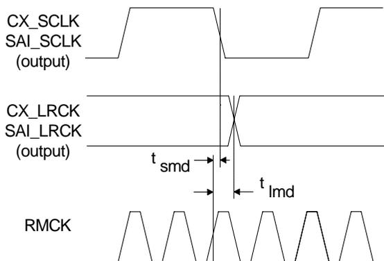
**Figure 1. Serial Audio Port Master Mode Timing**
