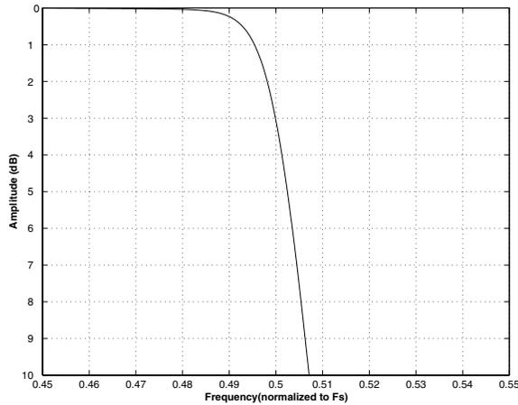
**Figure 47. Single Speed (fast) Transition Band (detail)**
