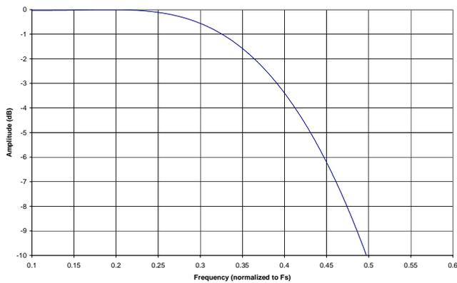
**Figure 43. Quad Speed Mode Transition Band (Detail)**
