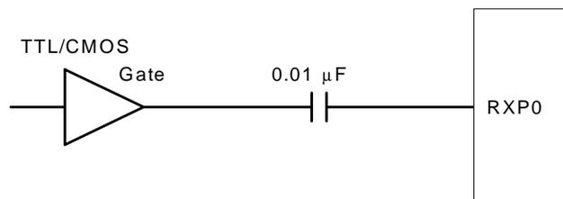
Figure 32. TTL/CMOS Input Circuit
