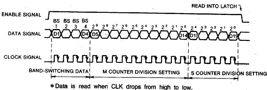
(2) When the control method selection pin SW is set to GND, the division ratio of the programmable divider and band-switching output is as shown below.
