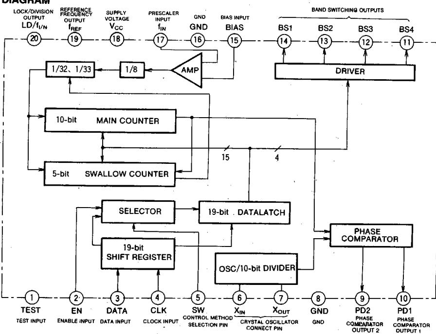
SERIAL INPUT PLL FREQUENCY SYNTHESIZER FOR VCR
