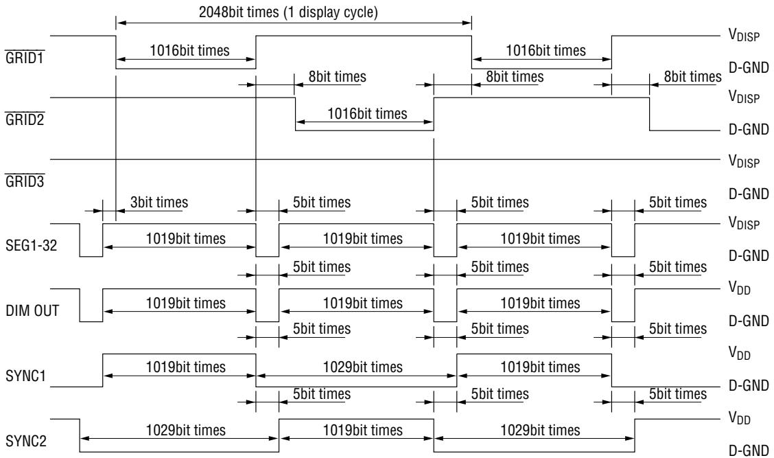
● **Output Timing (Triplex Operation)** \*1bit time=4x f<sub>OSC</sub>
