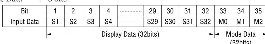
[Bit correspondence between segment output and display data]
