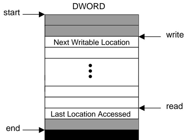
The empty queue states are illustrated in Figure 7. The queue is empty when the read index is one location before the write index, or when the read index is one location before the end index and the write index equals the start index.
