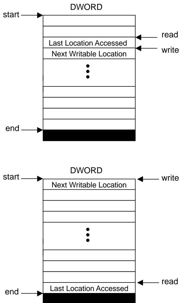
The full queue states are illustrated in Figure 8. The queue is full when the read index is equal to the write index.
