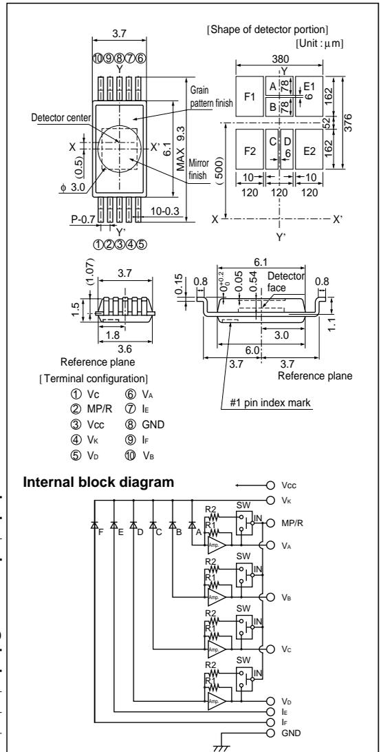
\* OPIC (Optical IC) is a trademark of the SHARP Corporation. An OPIC consists of a light-detecting element and signal-processing circuit integrated onto a single chip.
