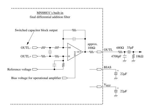
Structure of Analog Post Filter and Sample Analog Connections
