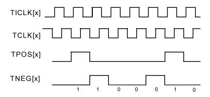
The Transmit Bipolar DS3 Stream diagram illustrates the generation of a bipolar DS3 stream. The B3ZS encoded DS3 stream is present on TPOS and TNEG. These outputs, along with the transmit clock, TCLK, can be directly connected to a DS3 line interface unit. Note that TCLK is a flow through version of TICLK; a variable propagation delay exists between these two signals.
