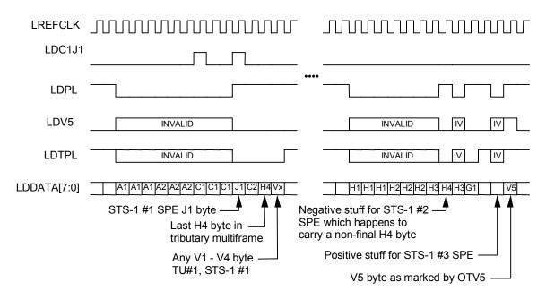
The LDV5 and LDTPL signals are optional when using the ingress VTPP within the TEMUX-84 which will regenerate the LDV5 and LDTPL signals from LDC1J1V1, LDPL and the pointers within LDDATA[7:0]. In order to bypass the ingress VTPP, the data on the Telecom drop bus must be locked such that all three STS-1 SPEs are aligned to the STS-3 transport envelope with the J1 bytes immediately following the C1 bytes. This is shown in Figure 59.
