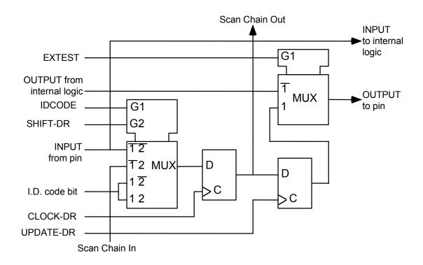
Figure 37 Layout of Output Enable and Bidirectional Cells
