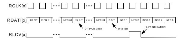
The Receive Unipolar DS3 Stream diagram (Figure 39) shows the complete DS3 receive signal on the RDAT input. Line code violation indications, detected by an upstream B3ZS decoder, are indicated on input RLCV. RLCV is sampled each bit period. The PMON Line Code Violation Event Counter is incremented each time a logic 1 is sampled on RLCV.
