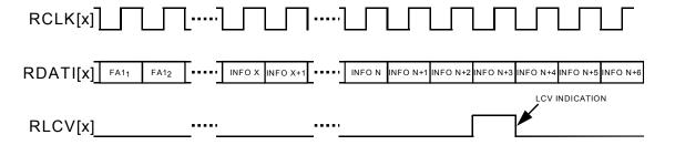
The Receive Unipolar E3 Stream diagram (Figure 41) shows the unipolar E3 receive signal on the RDATI[x] input. Line code violation indications, detected by an upstream HDB3 decoder, are indicated on input RLCV. RLCV is sampled each bit period. The PMON Line Code Violation Event Counter is incremented each time a logic 1 is sampled on RLCV.
