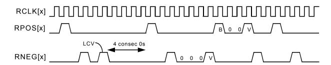
The Receive Bipolar E3 Stream diagram (Figure 40) shows the operation of the TEMUX-84 while processing an HDB3-encoded E3 stream on inputs RPOS[x] and RNEG[x]. It is assumed that the first bipolar violation (on RNEG[x]) illustrated corresponds to a valid HDB3 signature. A line code violation is declared upon detection of four consecutive zeros in the incoming stream, or upon detection of a bipolar violation which is not part of a valid HDB3 signature.
