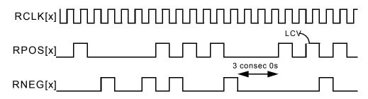
The Receive Bipolar DS3 Stream diagram (Figure 38) shows the operation of the TEMUX-84 while processing a B3ZS encoded DS3 stream on inputs RPOS and RNEG. It is assumed that the first bipolar violation (on RNEG) illustrated corresponds to a valid B3ZS signature. A line code violation is declared upon detection of three consecutive zeros in the incoming stream, or upon detection of a bipolar violation which is not part of a valid B3ZS signature.
