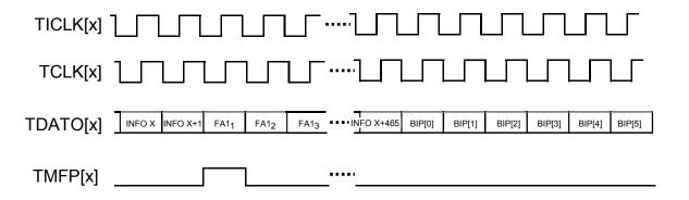
The Transmit Unipolar E3 Stream diagram (Figure 45) illustrates the unipolar E3 stream generation. The TMFP output shown marks the G.832 frame boundary (the first bit of the FA1 frame alignment byte) in the transmit stream. Note that TCLK is a flow through version of TICLK; a variable propagation delay exists between these two signals.
