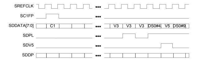
Figure 64 illustrates the operation of the SBI DROP Bus, using a negative justification on the second to last V3 octet as an example. The justification is indicated by asserting SDPL high during the V3 octet. The timing diagram also shows the location of one of the tributaries by asserting SDV5 high during the V5 octet.
