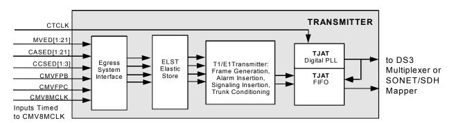
When Clock Slave: H-MVIP mode is enabled a 8.192 Mbit/s H-MVIP egress interface multiplexes up to 2016 channels from 84 T1s or 63 E1s, up to 2016 channel associated signaling (CAS) channels from 84 T1s or 63 E1s and common channel signaling from up to 84 T1s or 63 E1s. The H-MVIP interfaces use common clocks, CMV8MCLK and CMVFPC, and frame pulse, CMVFPB, for synchronization.
