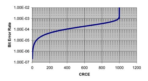
Figure 20 illustrates the expected count values for a range of Bit Error Ratios in T1 mode.
