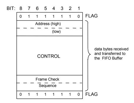
Bit 1 is the first serial bit to be received. When enabled, the primary, secondary and universal addresses are compared with the high order packet address to determine a match.
