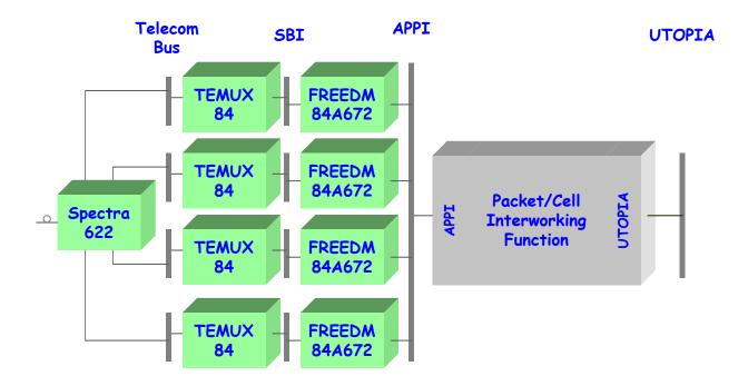
HIGH DENSITY T1/E1 FRAMER WITH INTEGRATED VT/TU MAPPER AND M13 MUX
