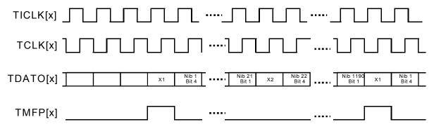
The Transmit Unipolar DS3 Stream diagram (Figure 43) illustrates the unipolar DS3 stream generation. The TMFP output marks the M-frame boundary, X1 bit, in the transmit stream. Note that TCLK is a flow through version of TICLK; a variable propagation delay exists between these two signals.
