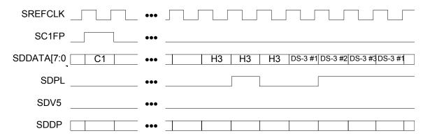
Figure 65 shows three DS-3 tributaries mapped onto the SBI bus. A negative justification is shown for DS-3 #2 during the H3 octet with SDPL asserted high. A positive justification is shown for DS-3#1 during the first DS-3#1 octet after H3 which has SDPL asserted low. E3 is transported by the same mechanism.
