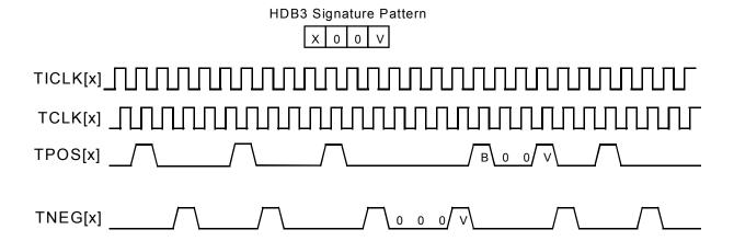
The Transmit Bipolar E3 Stream diagram (Figure 44) illustrates the generation of a bipolar E3 stream. The HDB3 encoded E3 stream is present on TPOS and TNEG. These outputs, along with the transmit clock, TCLK, can be directly connected to a E3 line interface unit. Note that TCLK is a flow through version of TICLK; a variable propagation delay exists between these two signals.
