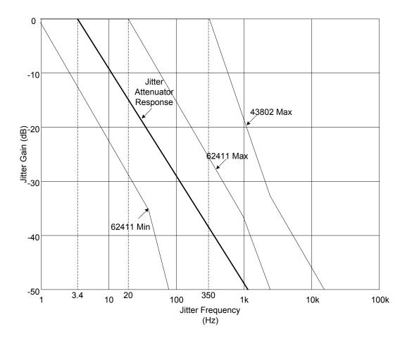
The output jitter in E1 mode for jitter frequencies from 0 to 5.0 Hz is no more than 0.1 dB greater than the input jitter, excluding the residual jitter. Jitter frequencies above 2.5 Hz are attenuated at a level of 20 dB per decade, as shown in Figure 13.
