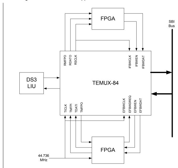
To support evolving fractional DS3 applications, flow-controlled ports provide access to SBI bus bandwidth. Several non-standard schemes have been devised to use a portion of the DS3 payload. Given that these protocols are subject to change, they are best supported by external programmable logic. Figure 3 illustrates one implementation. Other implementations and applications are possible.
