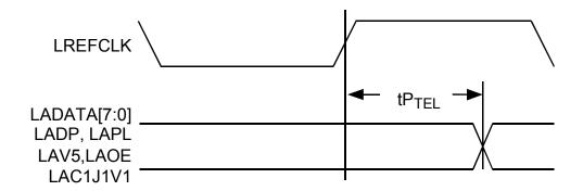
Figure 73 Telecom BUS Tristate Output Timing
