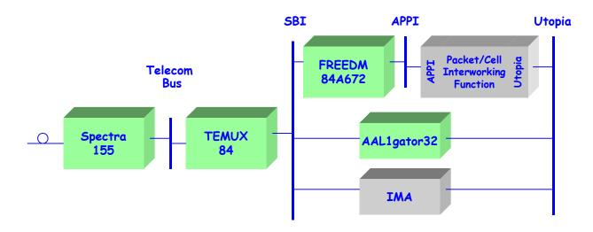
Figure 1illustrates how frame relay (FREEDM84A672), circuit emulation (AAL1gator32) and ATM inverse multiplexing (IMA84) may all be supported on the same port with a common SBI bus as the enabling technology.
