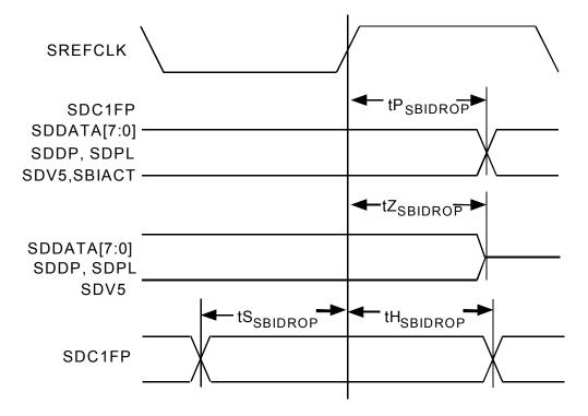
Figure 76 SBI DROP BUS Collision Avoidance Timing
