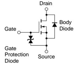
**Remark** The diode connected between the gate and source of the transistor serves as a protector against ESD.
