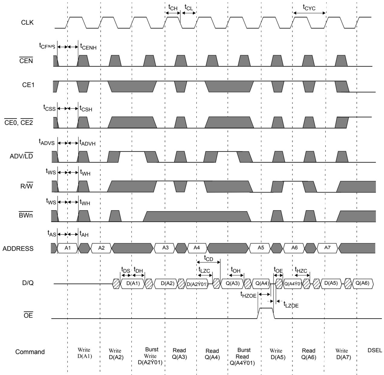
Note:  $\dot{Y}$  = XOR when  $\overline{LBO}$  = high/no connect.  $\dot{Y}$  = ADD when  $\overline{LBO}$  = low.  $\overline{BW[a:d]}$  is don't care.
