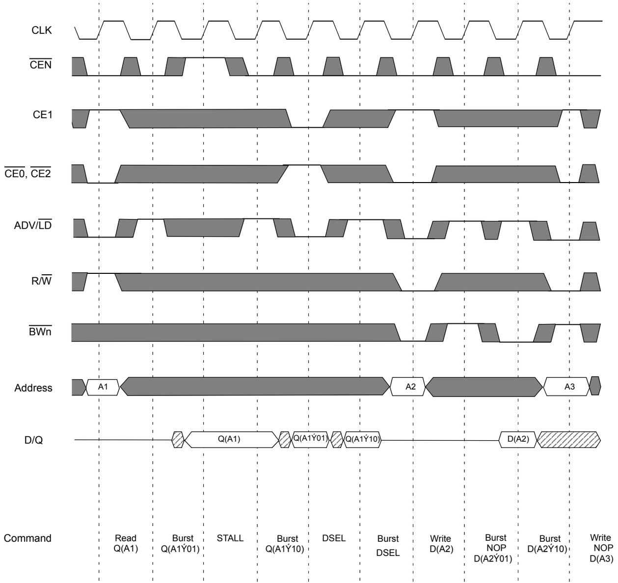
Note:  $\dot{Y}$  = XOR when  $\overline{LBO}$  = high/no connect;  $\dot{Y}$  = ADD when  $\overline{LBO}$  = low.  $\overline{OE}$  is low.
