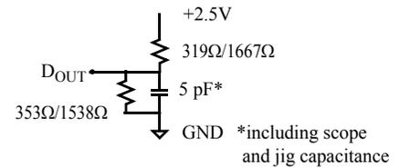
Figure C: Output load(B)
