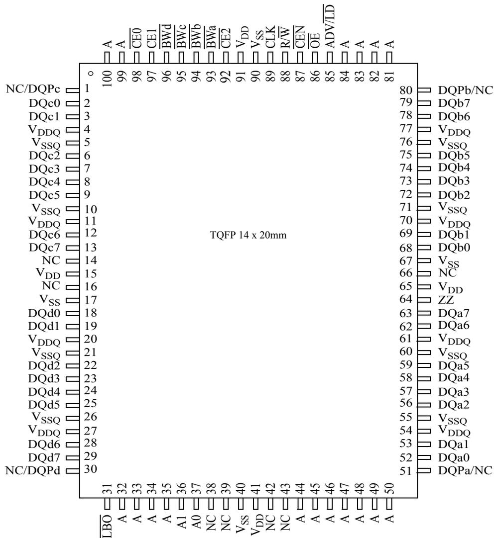
Note: For pins 1, 30, 51, and 80, NC applies to the x32 configuration. DQPn applies to the x36 configuration.
