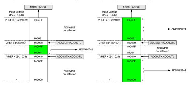
Figure 5.16. ADC Window Compare Example: Right-Justified Single-Ended Data
