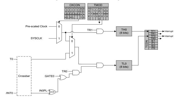
Figure 17.3. T0 Mode 3 Block Diagram
