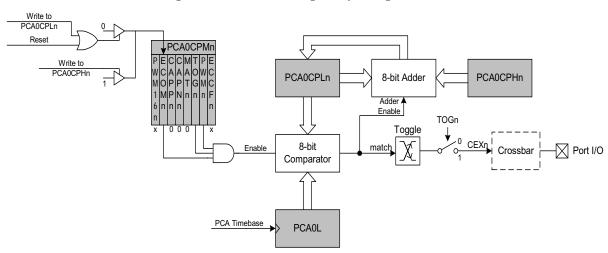
Figure 18.7. PCA Frequency Output Mode
