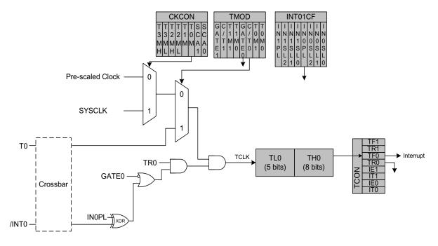
Figure 17.1. T0 Mode 0 Block Diagram
