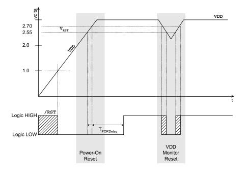
Figure 9.2. Power-On and VDD Monitor Reset Timing
