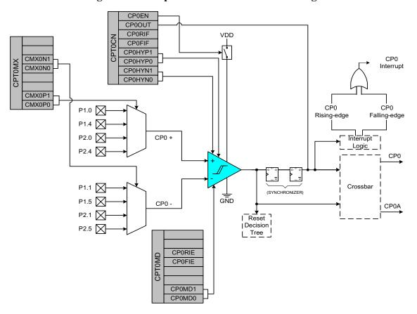
Figure 7.1. Comparator0 Functional Block Diagram
