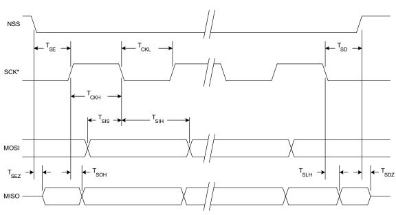
Figure 16.15. SPI Slave Timing (CKPHA = 1)
