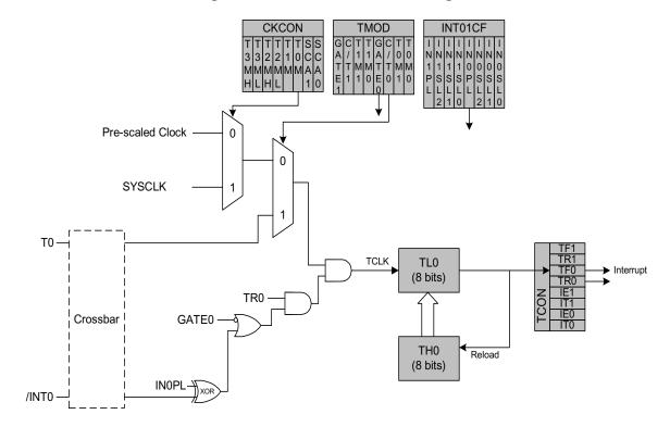
Figure 17.2. T0 Mode 2 Block Diagram
