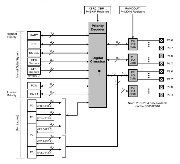
Figure 13.1. Port I/O Functional Block Diagram
