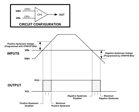
The Comparator hysteresis is software-programmable via its Comparator Control register CPTnCN (for n = 0 or 1). The user can program both the amount of hysteresis voltage (referred to the input voltage) and the positive and negative-going symmetry of this hysteresis around the threshold voltage.
