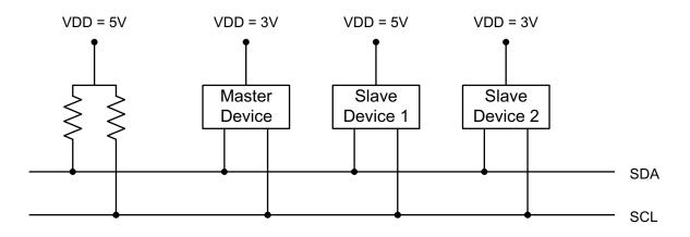
Figure 14.2. Typical SMBus Configuration
