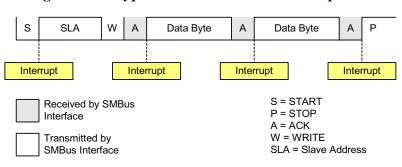
Figure 14.8. Typical Master Transmitter Sequence
