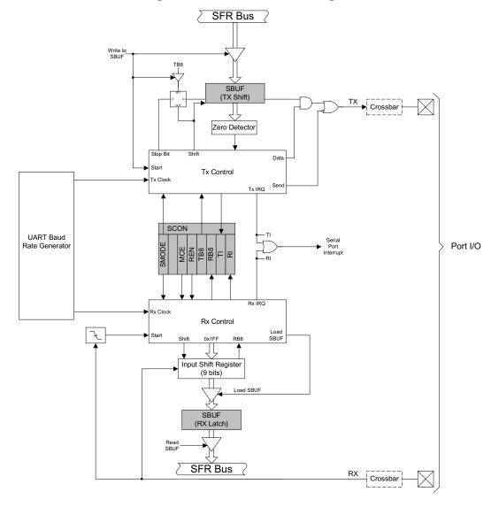
Figure 15.1. UARTO Block Diagram
