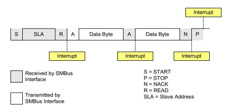
Figure 14.11. Typical Slave Transmitter Sequence
