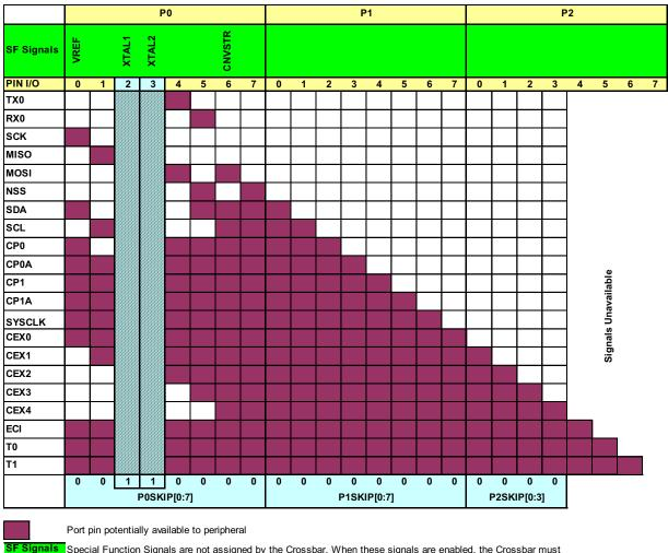
Figure 13.4. Crossbar Priority Decoder with Crystal Pins Skipped
