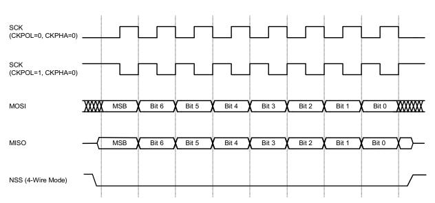
Figure 16.6. Slave Mode Data/Clock Timing (CKPHA = 0)
