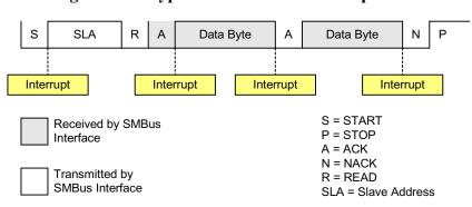
Figure 14.9. Typical Master Receiver Sequence
