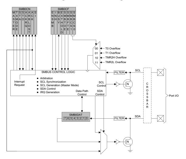
Figure 14.1. SMBus Block Diagram
