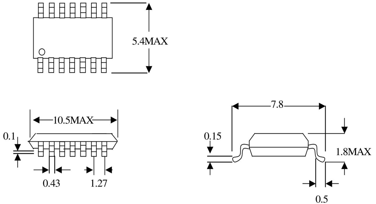
Note ) Lead pitch is 1.27 and tolerance is  $\pm 0.12$  against theoretical center of each lead that is obtain on the basis of No.1 and No.14 leads.
