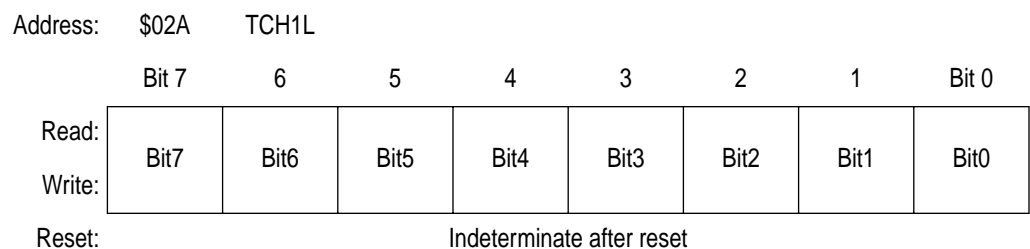
Figure 10-9. TIM Channel Registers (TCH0H/L:TCH1H/L)
