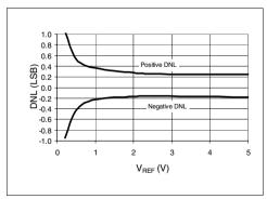
**FIGURE 2-9:** Differential Nonlinearity (DNL) vs.  $V_{REF.}$
