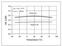
**FIGURE 2-10:** Integral Nonlinearity (INL) vs. Temperature ( $V_{DD} = 2.7V$ ).
