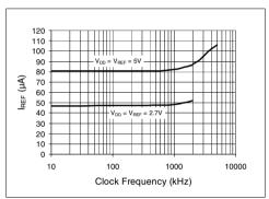
FIGURE 2-35: I<sub>REF</sub> vs. Clock Frequency.
