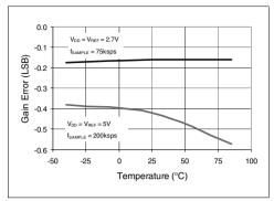
FIGURE 2-19: Gain Error vs. Temperature.
