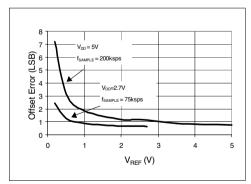
FIGURE 2-18: Offset Error vs. V<sub>REE</sub>.
