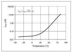
FIGURE 2-38: I<sub>DDS</sub> vs. Temperature.
