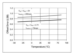
FIGURE 2-22: Offset Error vs. Temperature.
