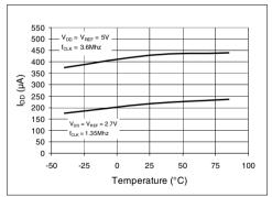
FIGURE 2-33: I<sub>DD</sub> vs. Temperature.
