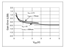
FIGURE 2-15: Gain Error vs. V<sub>REE</sub>.
