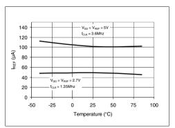
FIGURE 2-36: I<sub>REF</sub> vs. Temperature.
