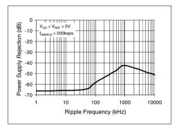
FIGURE 2-29: Power Supply Rejection (PSR) vs. Ripple Frequency.
