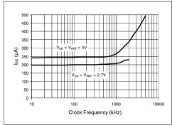
FIGURE 2-32: I<sub>DD</sub> vs. Clock Frequency.
