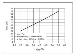
FIGURE 2-34: I<sub>REF</sub> vs. V<sub>DD.</sub>
