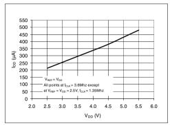
FIGURE 2-31: I<sub>DD</sub> vs. V<sub>DD.</sub>
