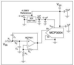
**FIGURE 6-3:** The MCP601 Operational Amplifier is used to implement a 2nd order anti-aliasing filter for the signal being converted by the MCP3004.
