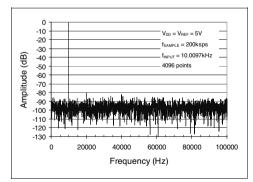
FIGURE 2-27: Frequency Spectrum of 10kHz input (Representative Part).
