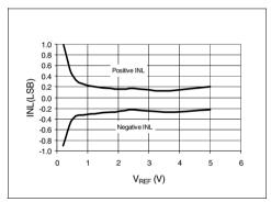
FIGURE 2-2: Integral Nonlinearity (INL) vs. V<sub>REF.</sub>
