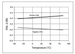
**FIGURE 2-14:** Differential Nonlinearity (DNL) vs. Temperature.
