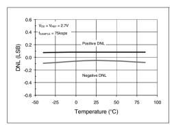
**FIGURE 2-17:** Differential Nonlinearity (DNL) vs. Temperature ( $V_{DD} = 2.7V$ ).
