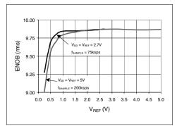
**FIGURE 2-25:** Effective Number of Bits (ENOB) vs.  $V_{REF.}$
