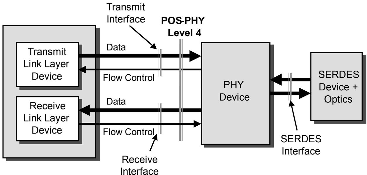
On both the transmit and receive interfaces, FIFO status information is sent separately from the corresponding data path. By taking FIFO status information out-of-band, it is possible to decouple the transmit and receive interfaces so that each operates independently of the other. Such an arrangement makes POS-PHY L4 suitable not only for bidirectional but also for unidirectional link layer devices.
