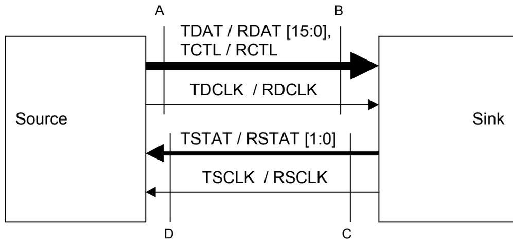
**Figure 2.14 Reference Points for Data Path Timing Parameters.**
