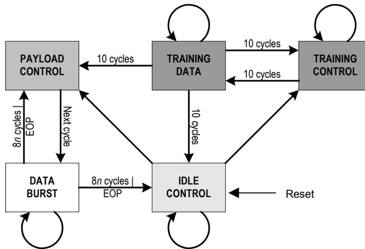
Figure 2.3 shows per-port state transitions at control word boundaries. At any given time, a given port may be active (sending data), paused (not sending data, but pending the completion of an outstanding packet), or inactive (not sending data, no outstanding packet).
