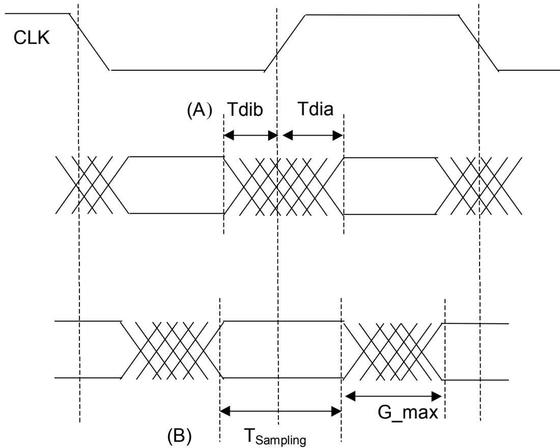
**Figure 2.15 Reference Points for FIFO Status Path Timing Parameters.**
