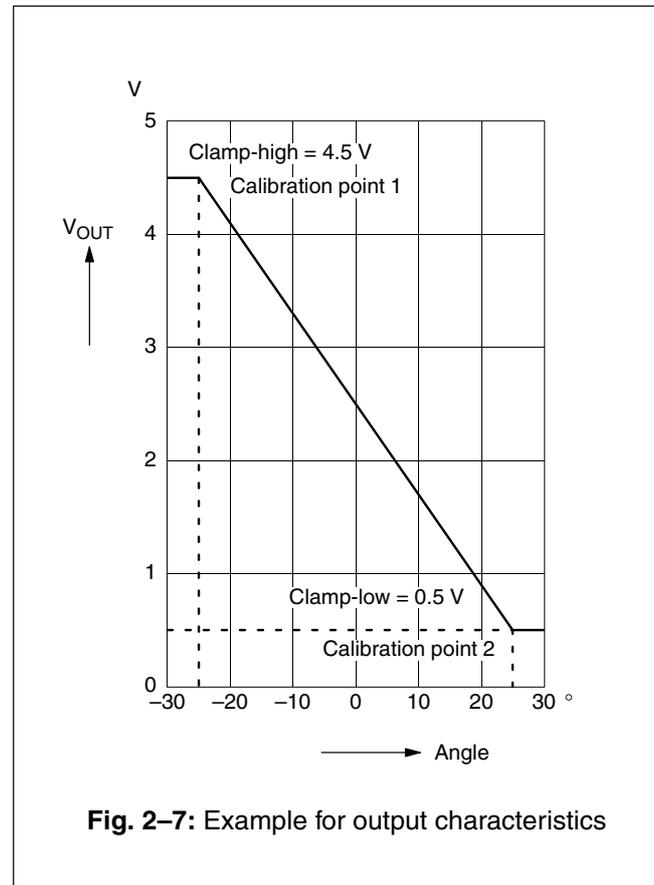
**Fig. 2-7: Example for output characteristics**
