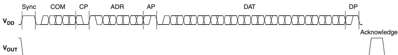
**Fig. 5-2:** Telegram for coding a Write command
