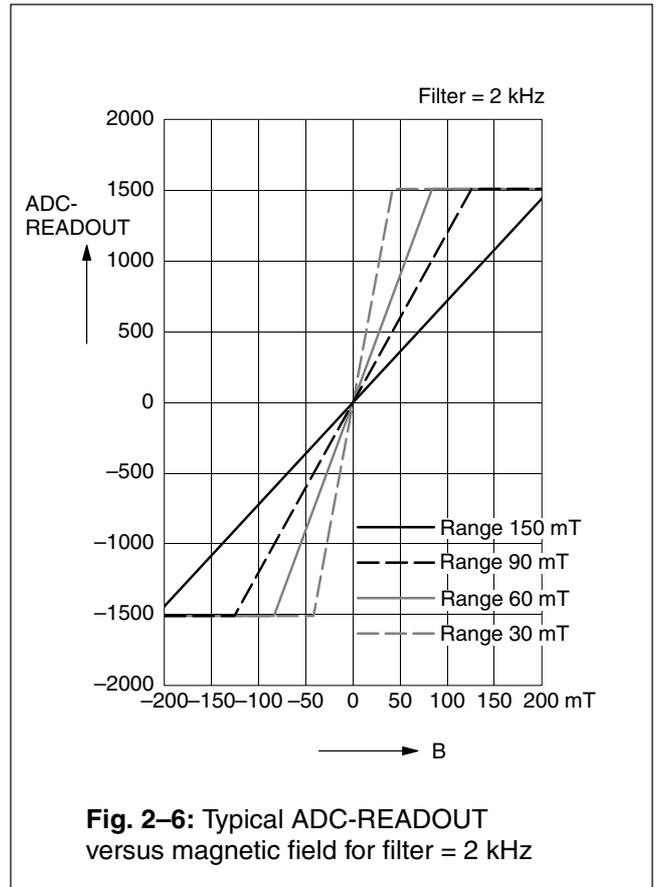
**Fig. 2–6:** Typical ADC-READOUT versus magnetic field for filter = 2 kHz
