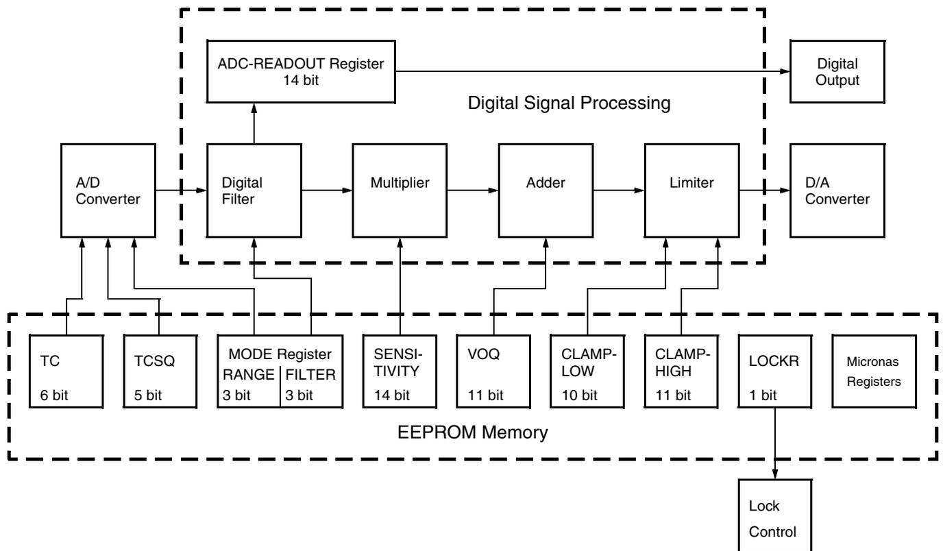
Fig. 2-3: Details of EEPROM and Digital Signal Processing
