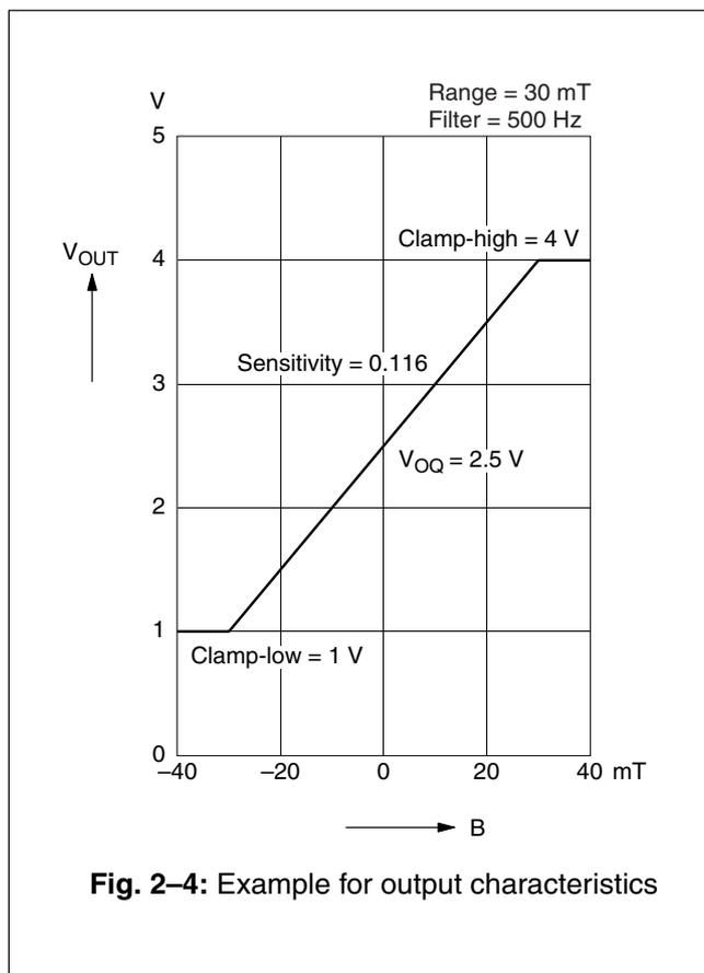
Fig. 2-4: Example for output characteristics
