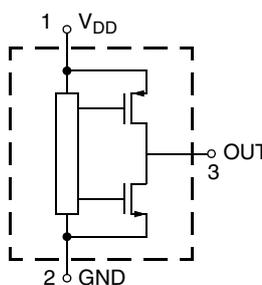
**Fig. 1–1:** Pin configuration
