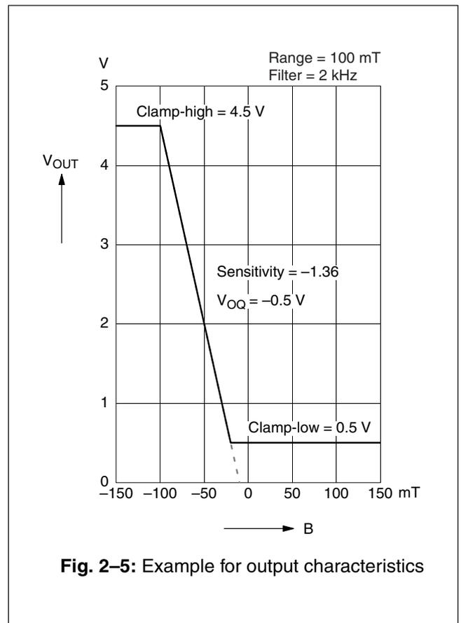
Fig. 2-5: Example for output characteristics
