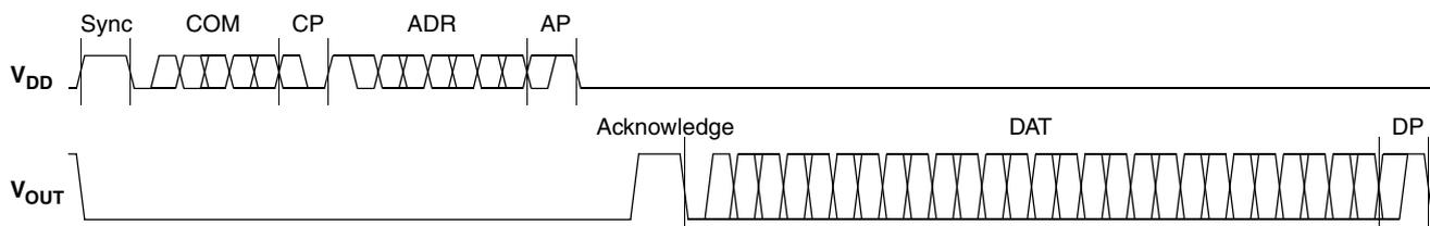
**Fig. 5-3:** Telegram for coding a Read command
