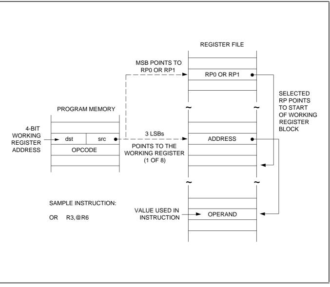
Figure 3–5. Indirect Working Register Addressing to Register File
