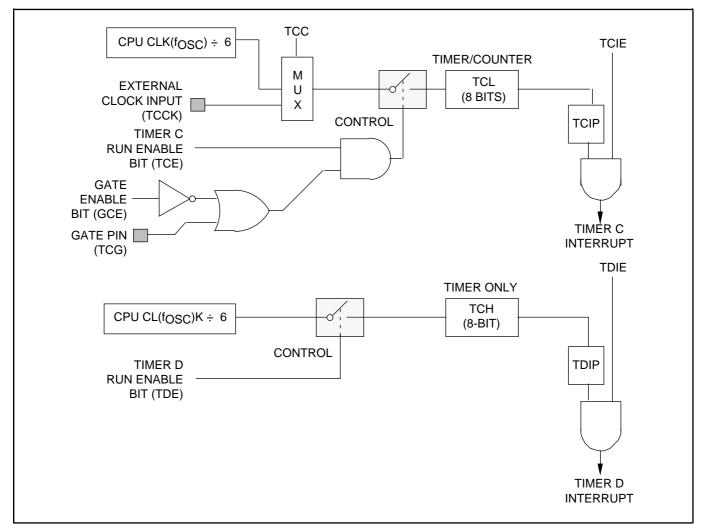
Figure 11–9. Timer Module 1 Mode 3 Function Diagram
