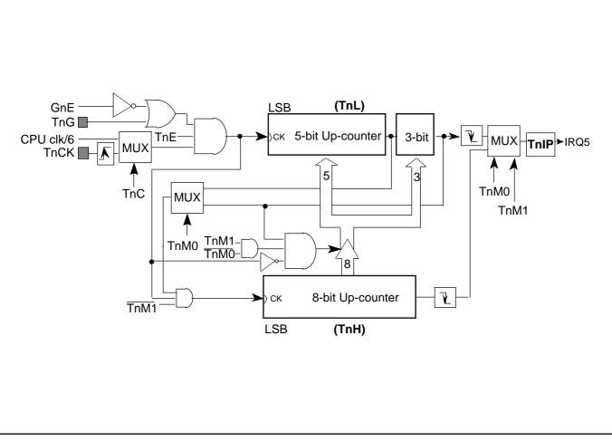
Figure 11-3. Timer C & D Block Diagram (MODE0–MODE2)
