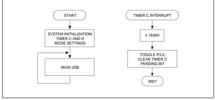
Figure 11–10. Timer Module 1 Mode 0 Programming Tip Flowchart
