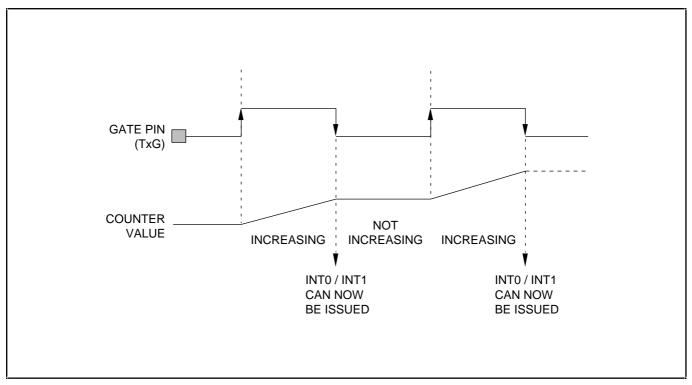
Figure 11–5. Count Value Incrementing With Gate Function Enabled
