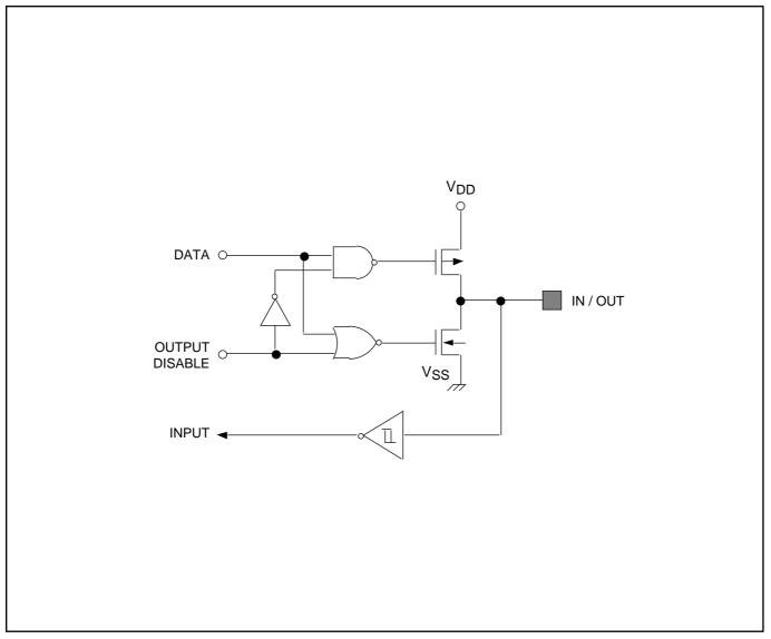
Figure 1–13. Pin Circuit Type 9 (Port AD)
