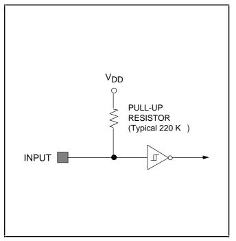
Figure 1–5. Pin Circuit Type 1 (RESET)
