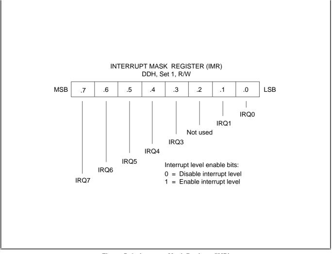
Figure 5–6. Interrupt Mask Register (IMR)
