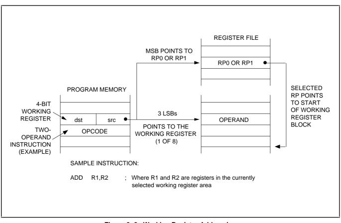
Figure 3–2. Working Register Addressing
