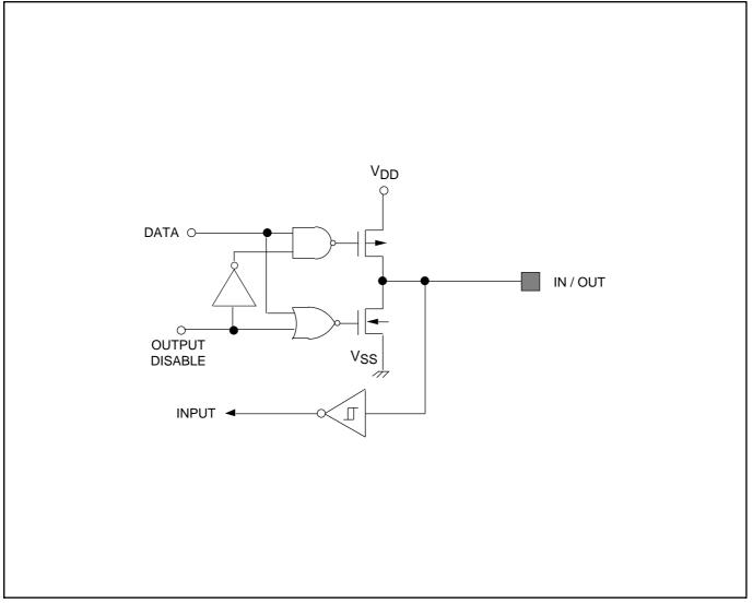
Figure 1–9. Pin Circuit Type 5 (P2.6/TA and P2.7/TB)
