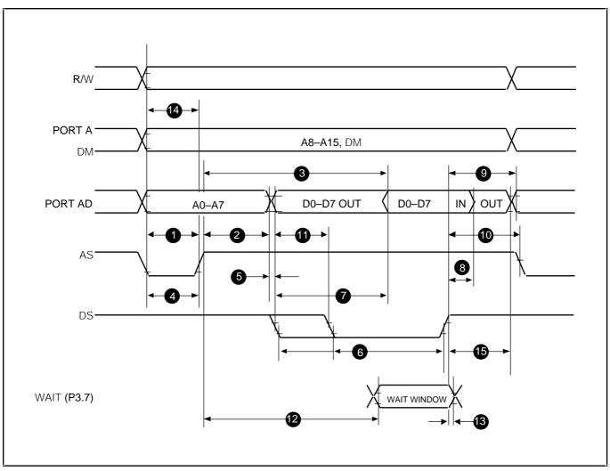
Figure 16–6. External Memory Read and Write Timing
