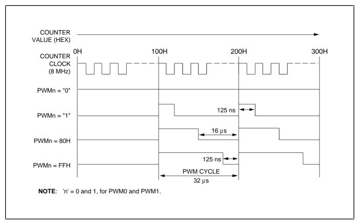
Figure 13–2. PWM Output Waveform and Timing Diagram
