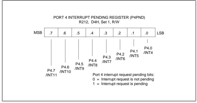
Figure 9–14. Port 4 Interrupt Pending Register (P4PND)\
