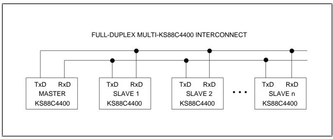
Figure 12–8. Connection Example for Multiprocessor Serial Data Communications
