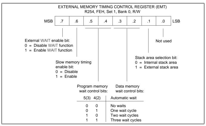
Figure 15–4. External Memory Timing Control Register (EMT)
