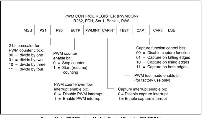
Figure 13–1. PWM/Capture Module Control Register (PWMCON)
