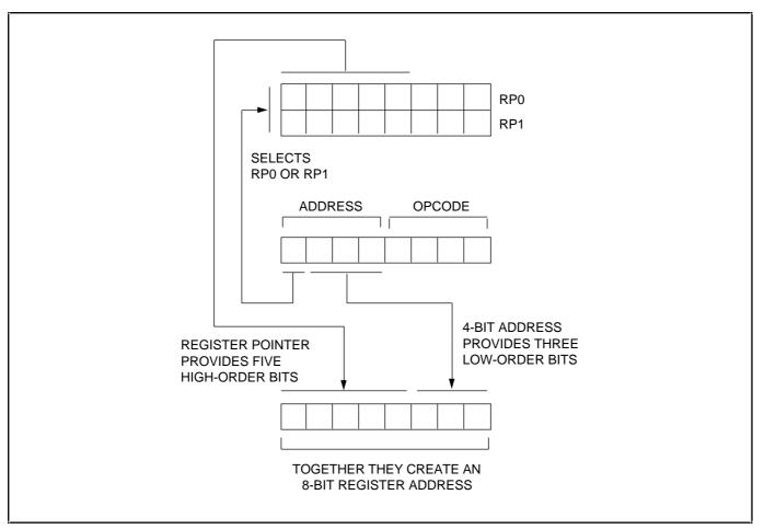
Figure 2–11. 4-Bit Working Register Addressing
