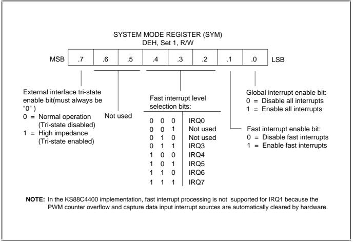
Figure 5–5. System Mode Register (SYM)
