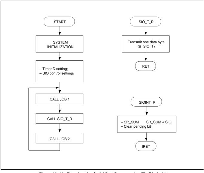
Figure 12–10. Flowchart for Serial Port Programming Tip (Mode 3)
