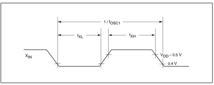
Figure 16–8. Clock Timing Measurement at XIN
