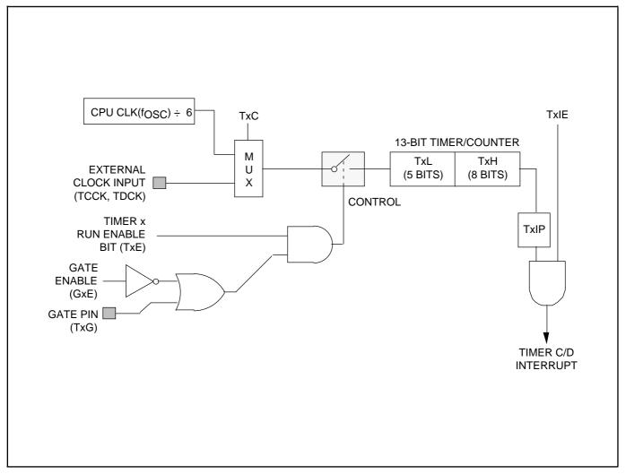
Figure 11–6. Timer Module 1 Mode 0 Function Diagram
