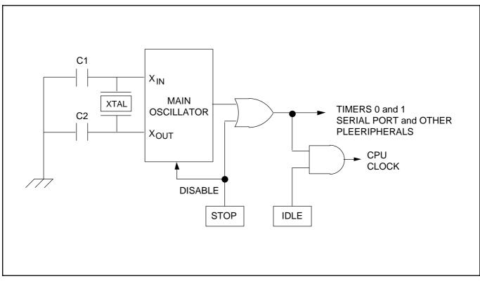
Figure 8–2. Stop and Idle Mode Function Diagram
