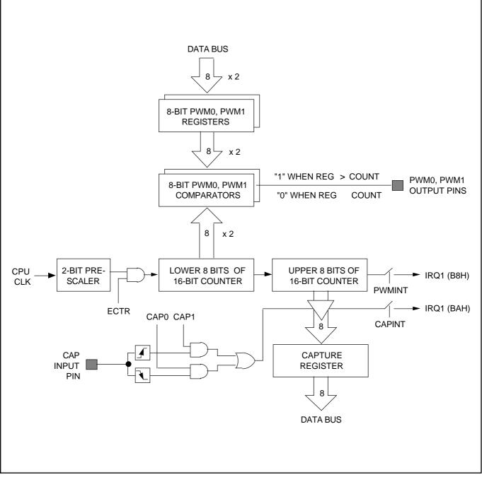
Figure 13–4. PWM/Capture Module Functional Block Diagram
