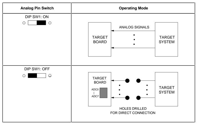
**NOTE**: Analog signals coming into the target board can easily introduce noise into the analog converter circuit. This can cause invalid conversion results. To reduce noise, you can use the analog pin switches to provide the shortest possible path for analog signals. To do this, turn all DIP switches to the OFF position. Then, connect the analog signal lines directly via the holes of the corresponding analog pins.
