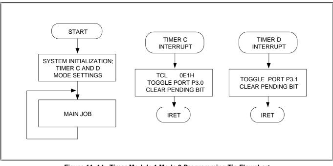
Figure 11–14. Timer Module 1 Mode 3 Programming Tip Flowchart
