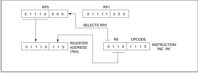
Figure 2–12. 4-Bit Working Register Addressing Example
