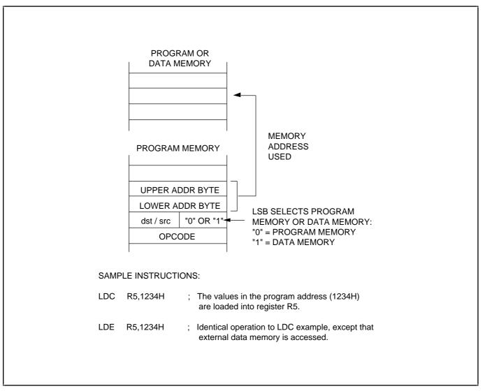
Figure 3–10. Direct Addressing for Load Instructions
