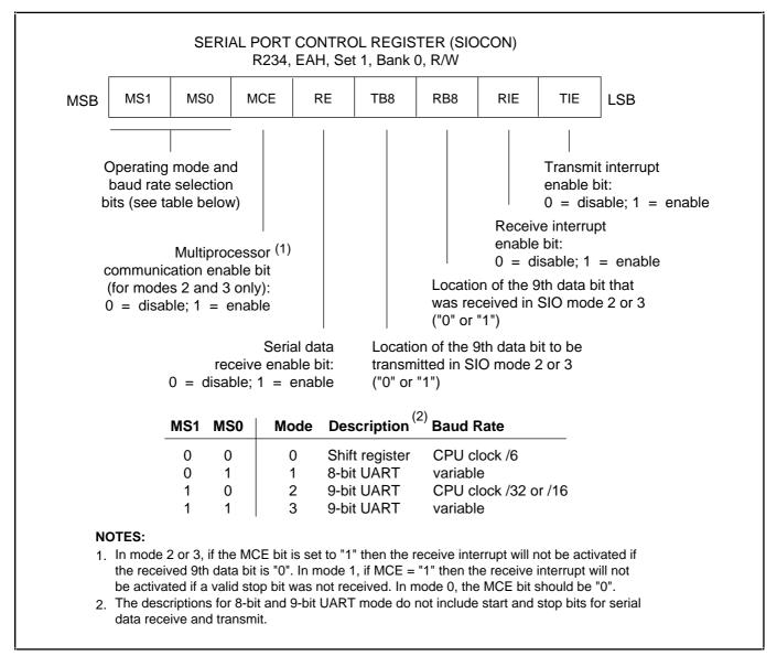
Figure 12–1. Serial Port Control Register (SIOCON)
