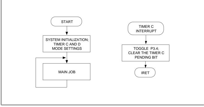
Figure 11–13. Timer Module 1 Mode 2 Programming Tip Flowchart
