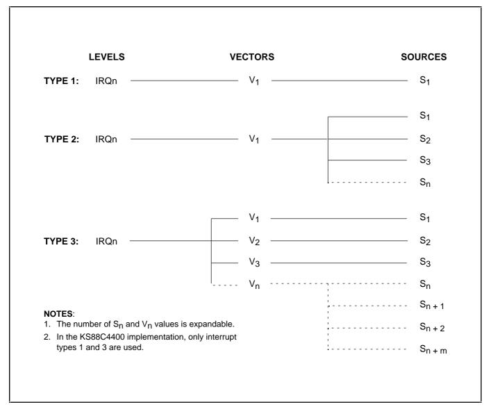
Figure 5–1. KS88-Series Interrupt Types
