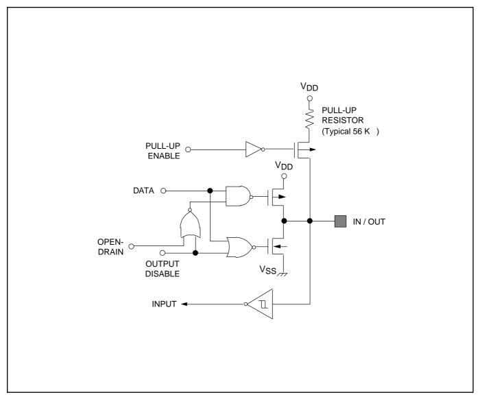
Figure 1–7. Pin Circuit Type 3 (Port 5)
