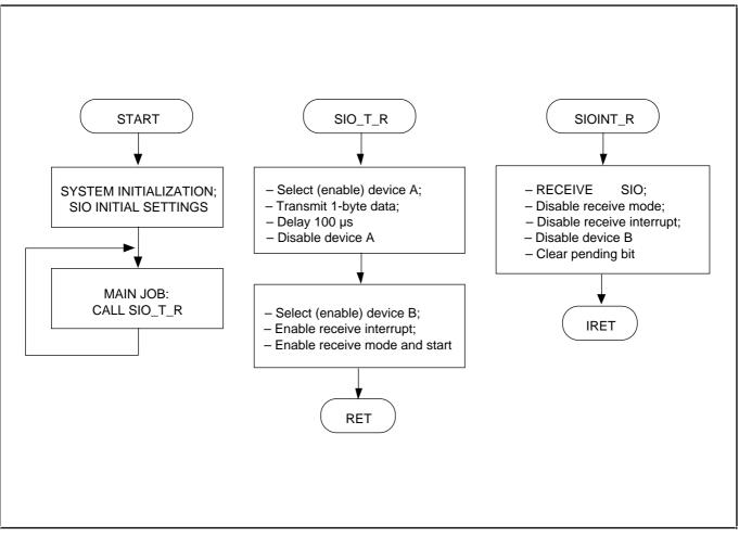
Figure 12–9. Flowchart for Serial Port Programming Tip (Mode 0)
