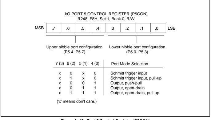
Figure 9–15. Port 5 Control Register (P5CON)
