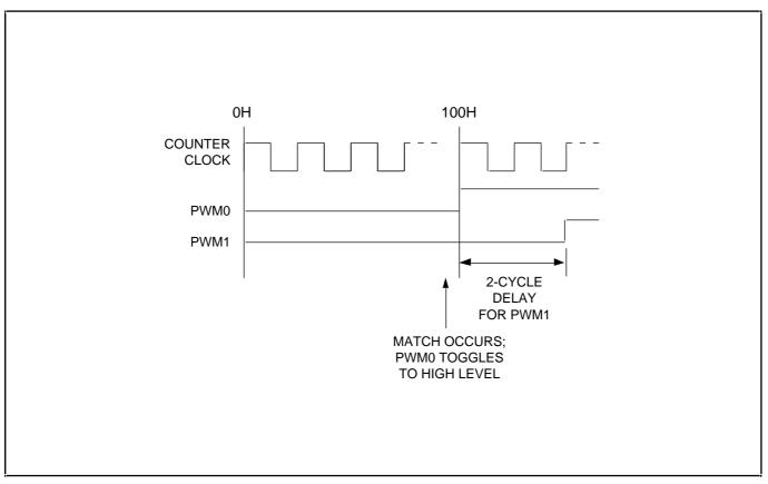
Figure 13–3. PWM0 and PWM1 Output Delay
