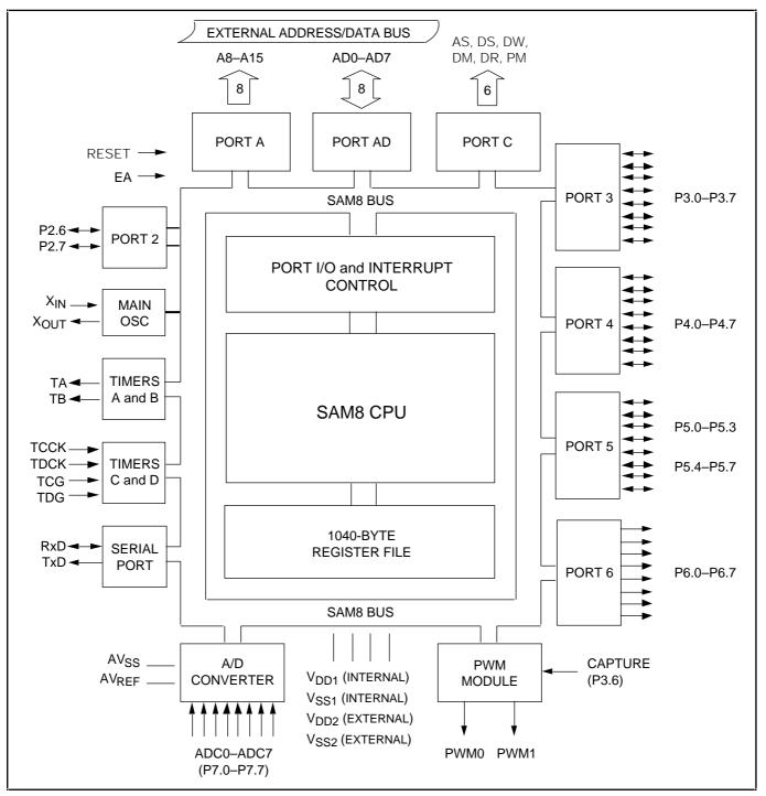
Figure 1–2. KS88C4400 Block Diagram
