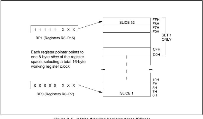
Figure 2–5. 8-Byte Working Register Areas (Slices)
