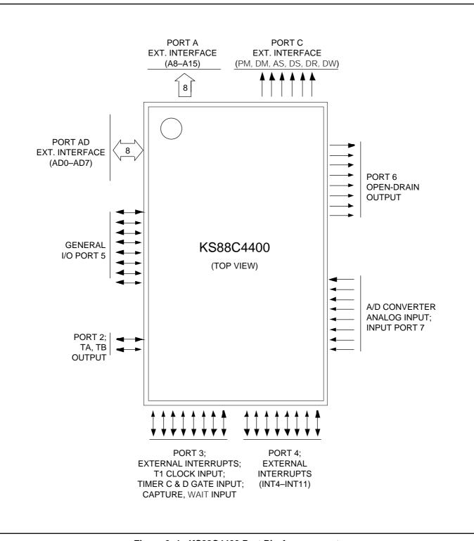
Figure 9–1. KS88C4400 Port Pin Arrangement
