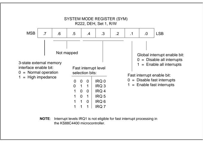
Figure 15–3. System Mode Register (SYM)
