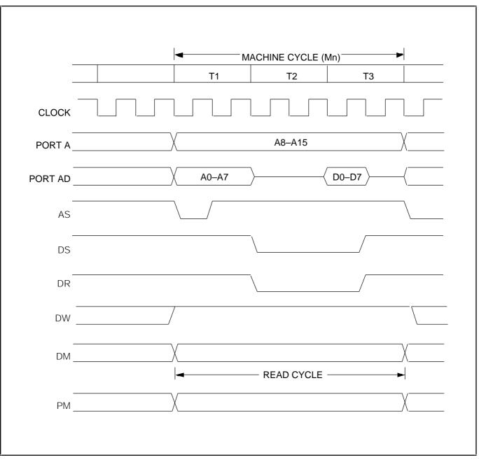
Figure 15–6. KS88C4400 External Bus Read Cycle Timing Diagram
