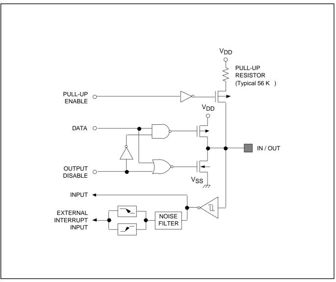
Figure 1–8. Pin Circuit Type 4 (Ports 3 and 4, TCCK, TDCK, TCG, TDG, CAP, WAIT, INT0–INT11)
