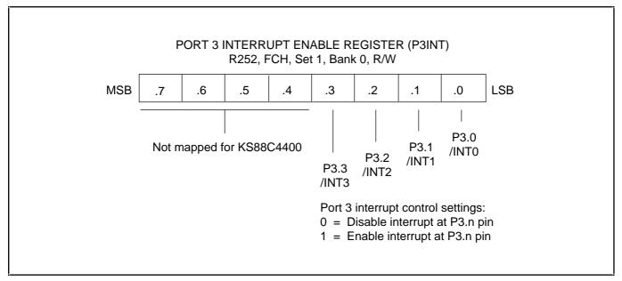
Figure 9–9. Port 3 Interrupt Enable Register (P3INT)
