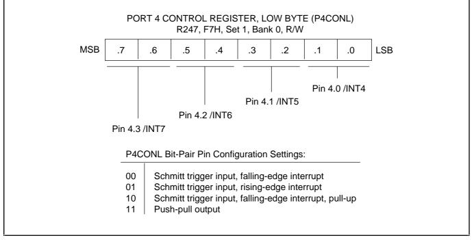
Figure 9–12. Port 4 Low-Byte Control Register (P4CONL)
