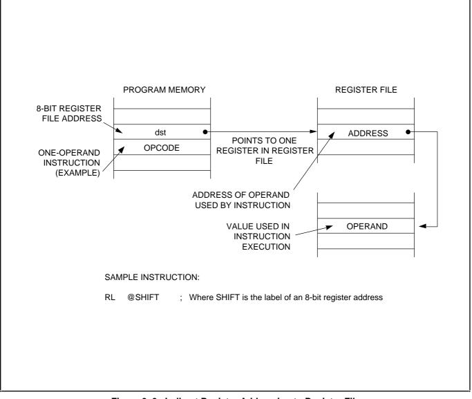
Figure 3–3. Indirect Register Addressing to Register File
