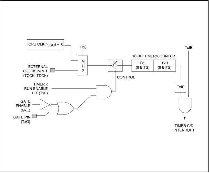
Figure 11–7. Timer Module 1 Mode 1 Function Diagram
