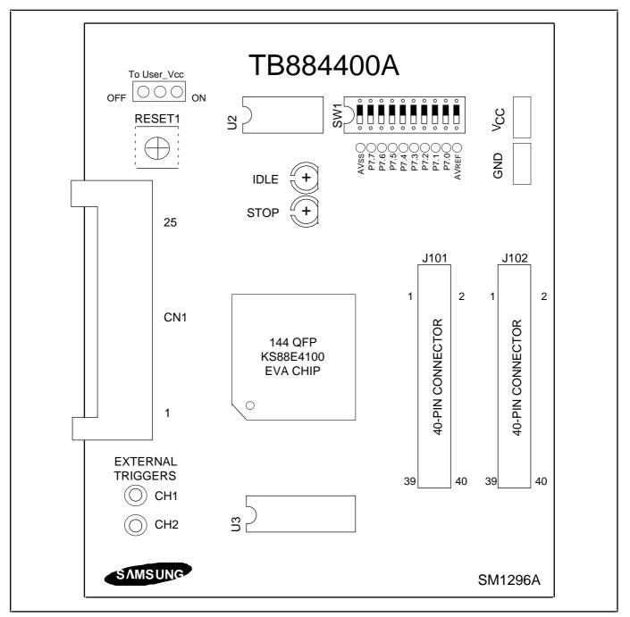
Figure 18–3. TB884400A Target Board Configuration
