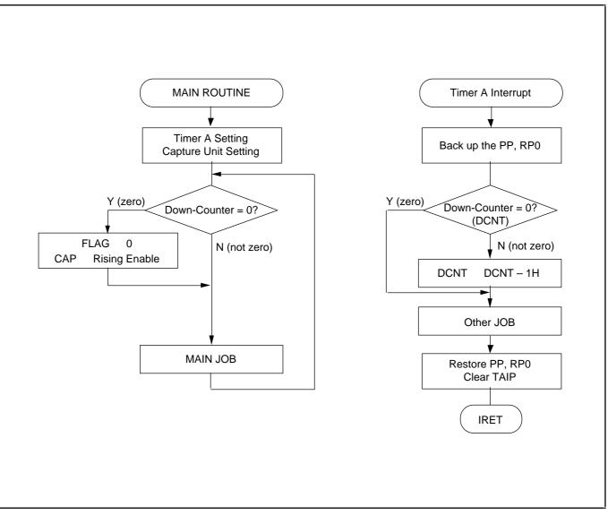
Figure 13–5. Decision Flowchart for Capture Unit Programming Tip
