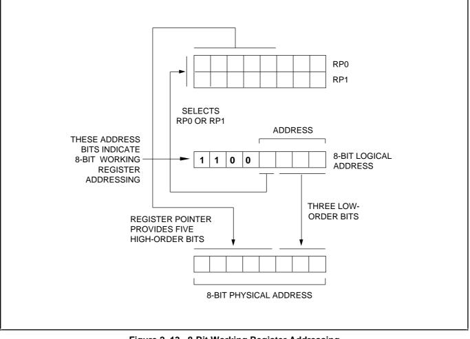
Figure 2–13. 8-Bit Working Register Addressing
