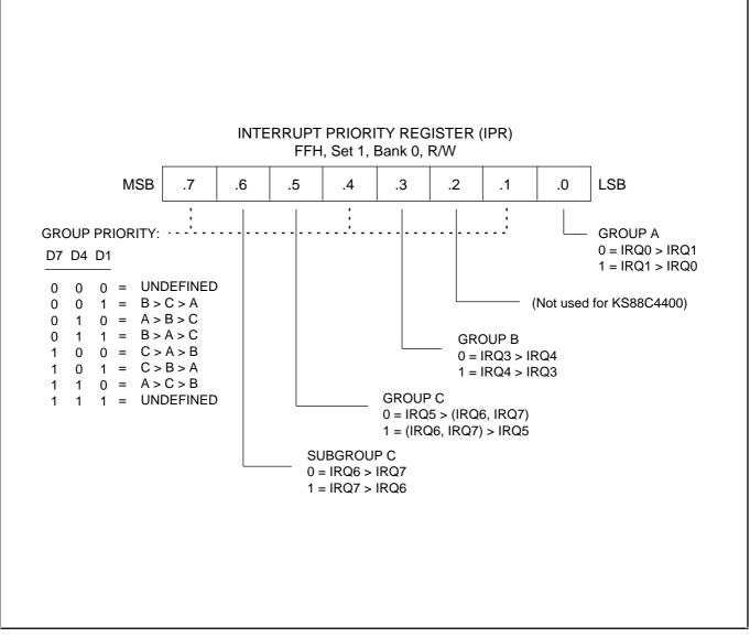
Figure 5–8. Interrupt Priority Register (IPR)
