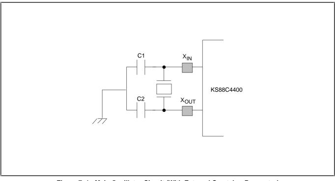
Figure 7–1. Main Oscillator Circuit (With External Crystal or Resonator)
