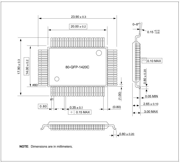
Figure 17–1. KS88C4400 QFP Standard Package Dimensions (in Millimeters)
