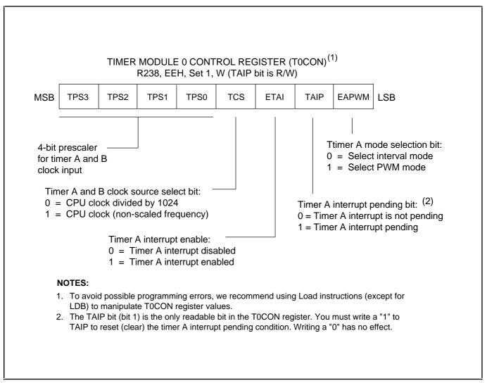
Figure 10–2. Timer Module 0 Control Register (T0CON)
