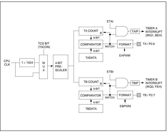
Figure 10–1. Timer Module 0 Function Block Diagram
