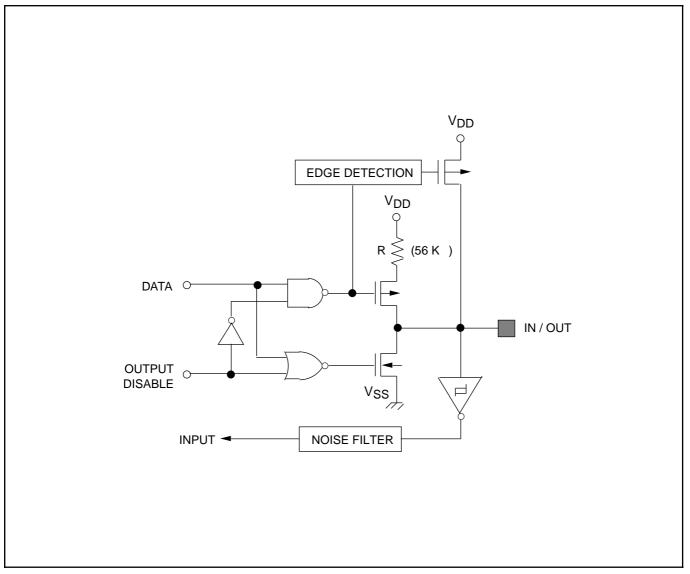
Figure 1–10. Pin Circuit Type 6 (Serial RxD Pin)
