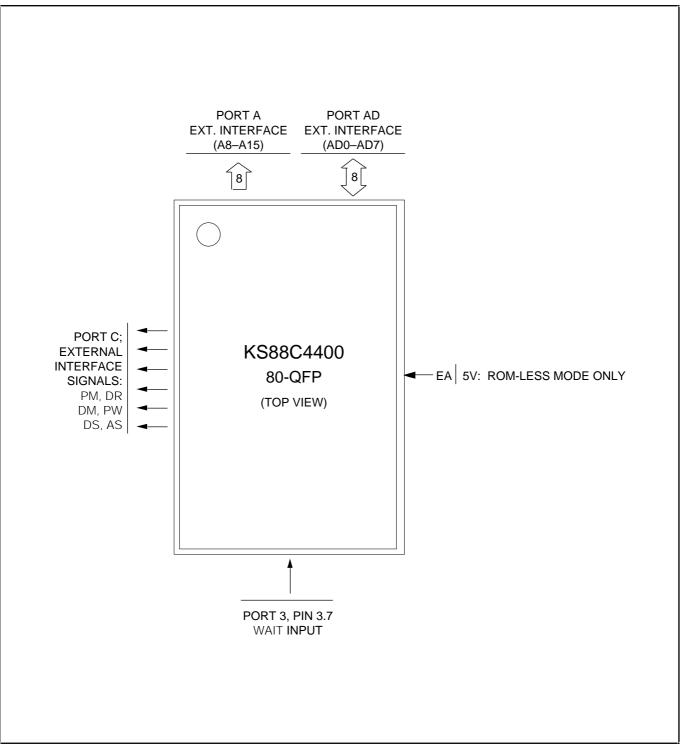
Figure 15–1. KS88C4400 Pin Functions for the External Interface
