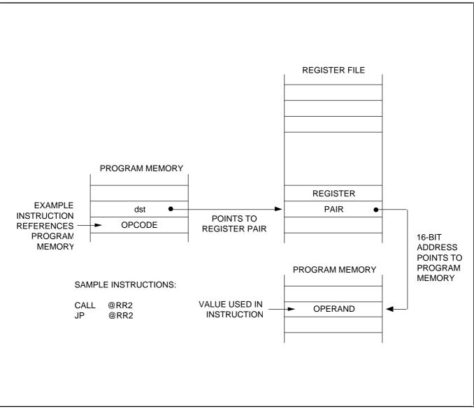
Figure 3–4. Indirect Register Addressing to Program Memory
