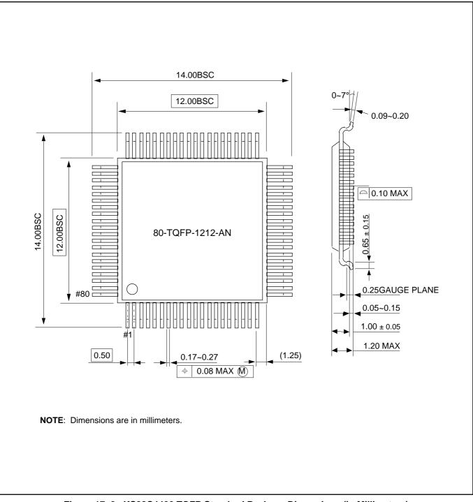
Figure 17–2. KS88C4400 TQFP Standard Package Dimensions (in Millimeters)
