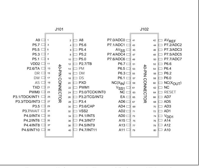
Figure 18–4. 40-Pin Connectors for TB884400A (KS88C4400, 80-QFP Package)
