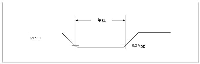
Figure 16–2. Input Timing for RESET
