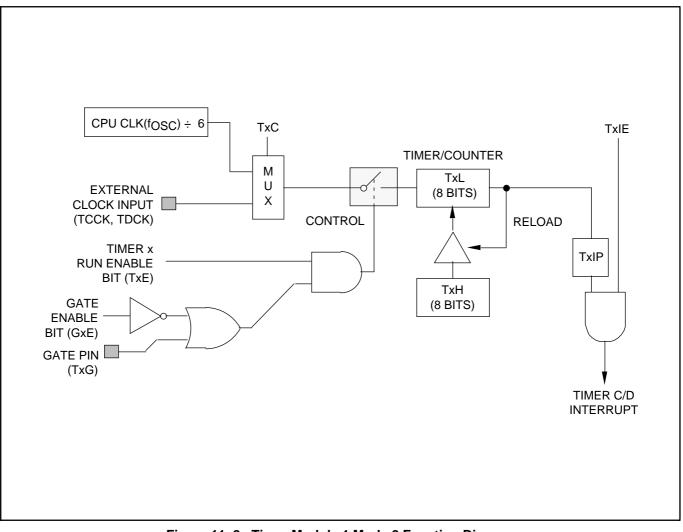
Figure 11–8. Timer Module 1 Mode 2 Function Diagram
