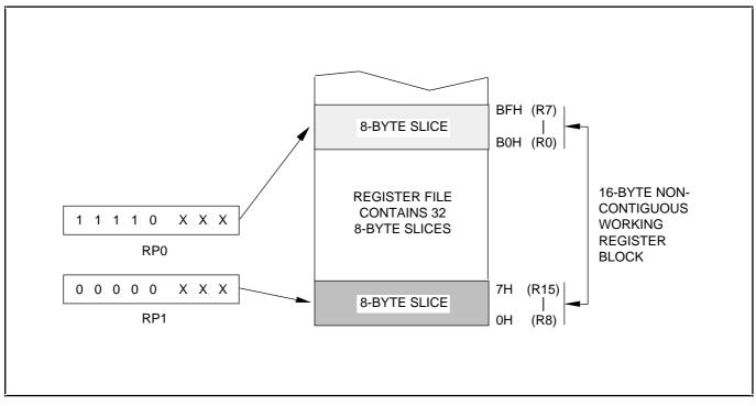
Figure 2–7. Non-Contiguous 16-Byte Working Register Block
