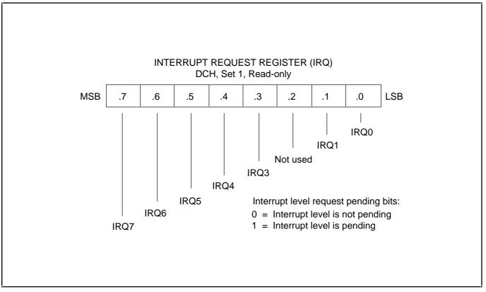
Figure 5–9. Interrupt Request Register (IRQ)
