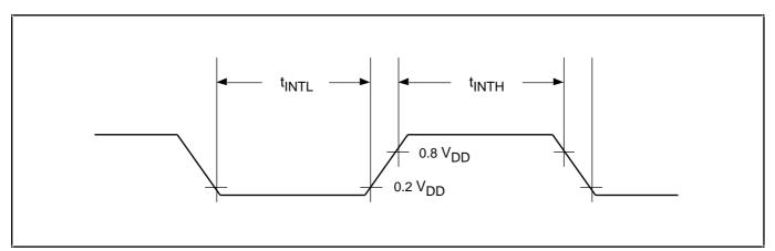
Figure 16–1. Input Timing for External Interrupts (Ports 3 and 4)
