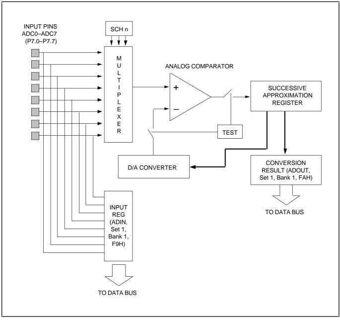
Figure 14–1. A/D Converter Functional Block Diagram
