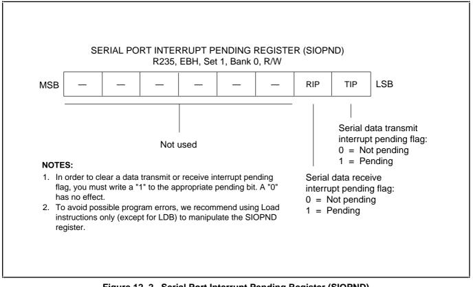
Figure 12–2. Serial Port Interrupt Pending Register (SIOPND)
