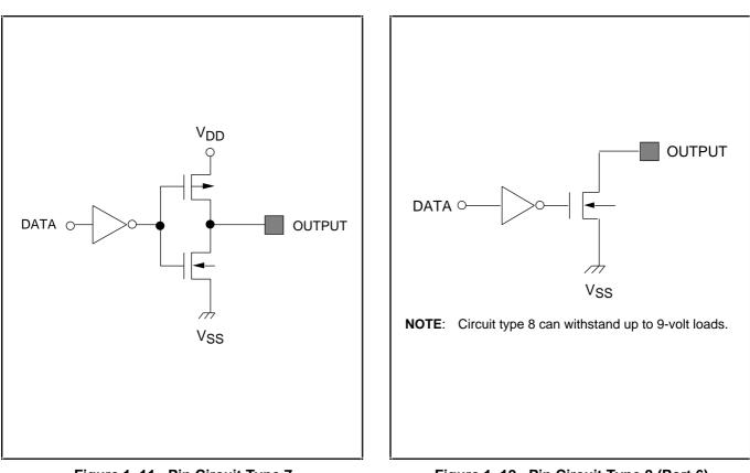
Figure 1–11. Pin Circuit Type 7 (Port A, port C, serial TxD Pin, PWM0, PWM1)
