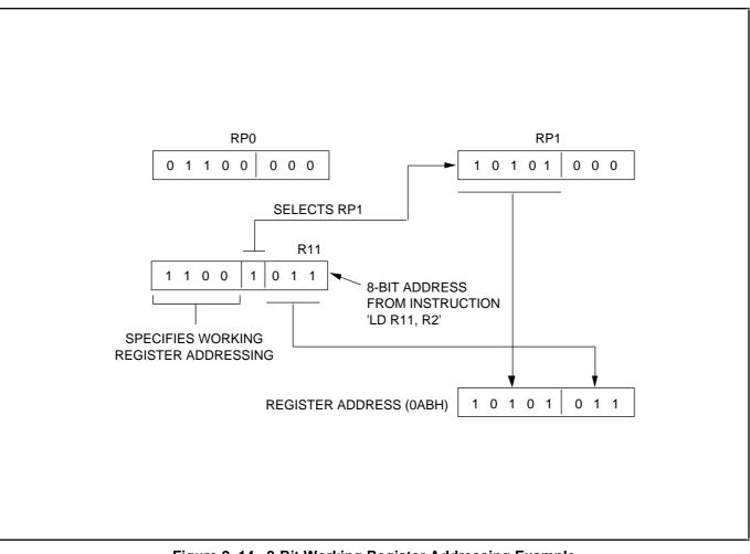
Figure 2–14. 8-Bit Working Register Addressing Example
