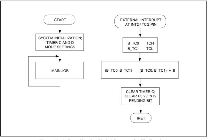
Figure 11–11. Timer Module 1 Mode 1 Programming Tip Flowchart
