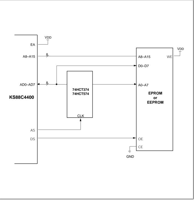
Figure 15–8. External Interface Function Diagram (External ROM Only)
