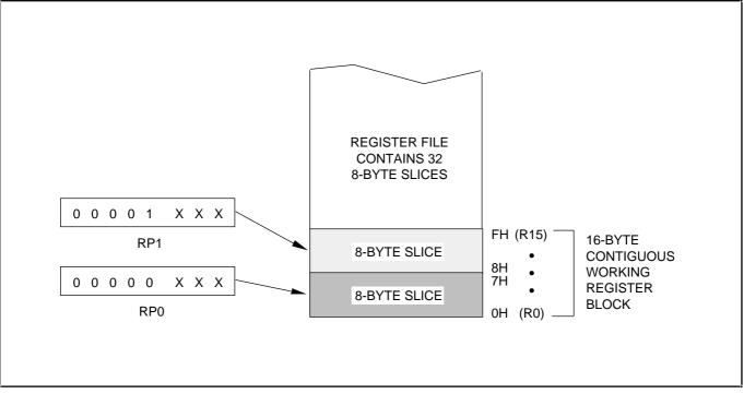
Figure 2–6. Contiguous 16-Byte Working Register Block
