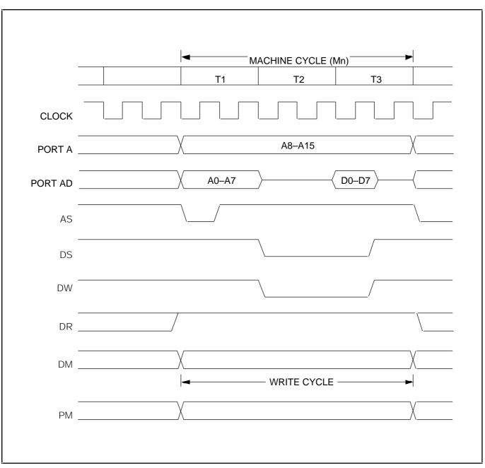
Figure 15–5. KS88C4400 External Bus Write Cycle Timing Diagram
