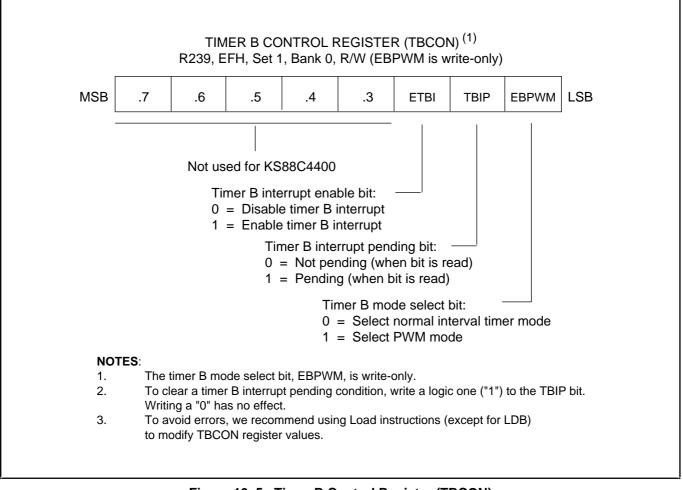
Figure 10–5. Timer B Control Register (TBCON)
