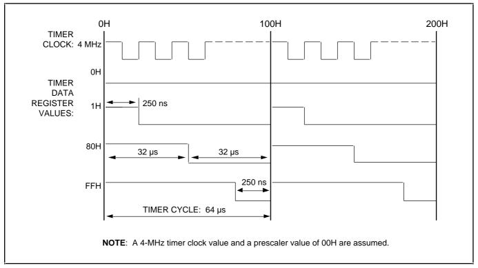
Figure 10–4. Timer A and B Waveforms in Pulse Width Modulation Mode
