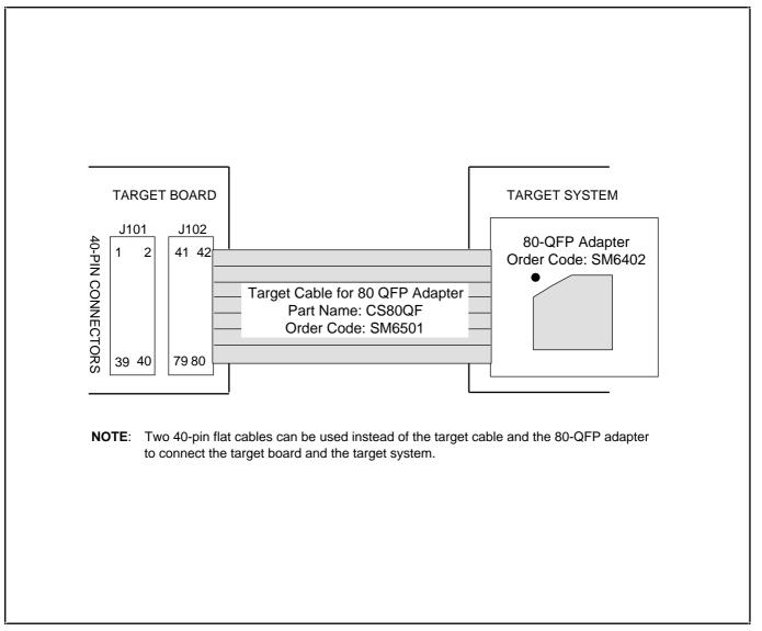
Figure 18–5. TB884400A Cable for 80-QFP Adapter
