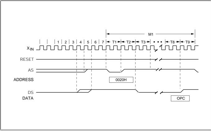
Figure 8–1. RESET Timing for External Interface (ROM-less Mode)
