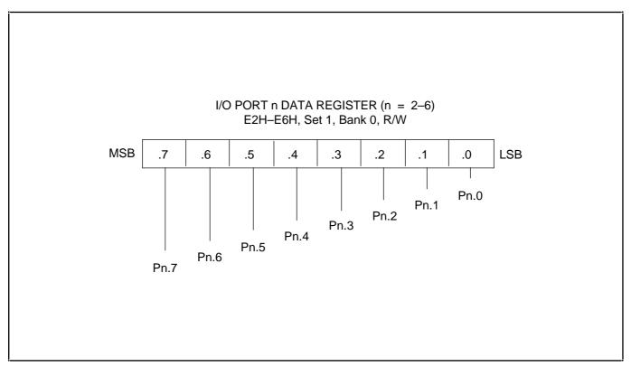
Figure 9–2. Port Data Register Structure
