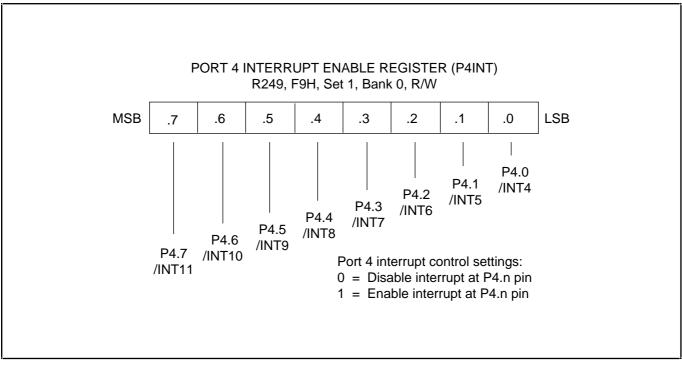
Figure 9–13. Port 4 Interrupt Enable Register (P4INT)
