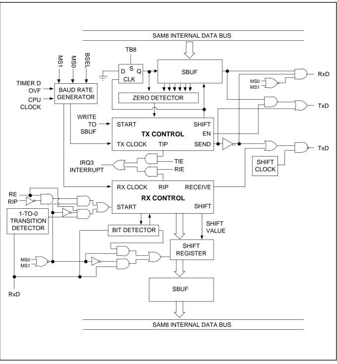
Figure 12–7. Serial Port (UART) Function Diagram
