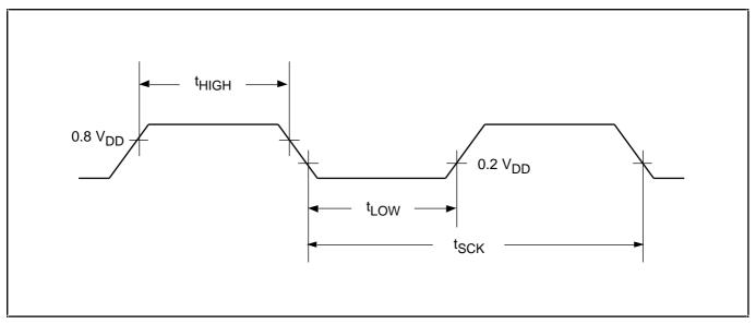
Figure 16–4. Serial Clock Waveform
