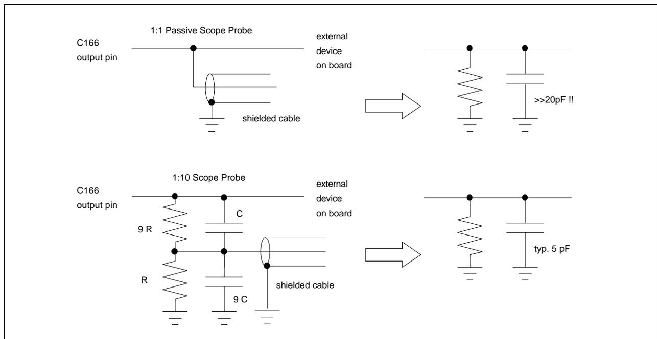
Different scope probes connected to signal lines influences the dynamic load of line drivers.
