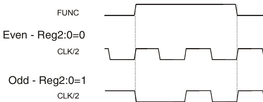
Figure 12-5 CLK/2: Even versus Odd
