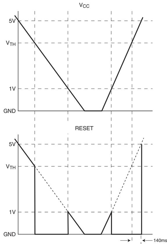
When operating properly with 5V  $V_{CC}$  (for example), /RESET will also be about 5V. When  $V_{CC}$  starts to fall, /RESET will follow it down as shown. When  $V_{CC}$  drops below  $V_{TH}$ , /RESET drops to ground ("issues a RESET") and stays there unless  $V_{CC}$  also falls below its minimum operating voltage, approx. 1V. At this point, the supervisor loses control, and its output may rise, only to again follow  $V_{CC}$  down to the ground.
