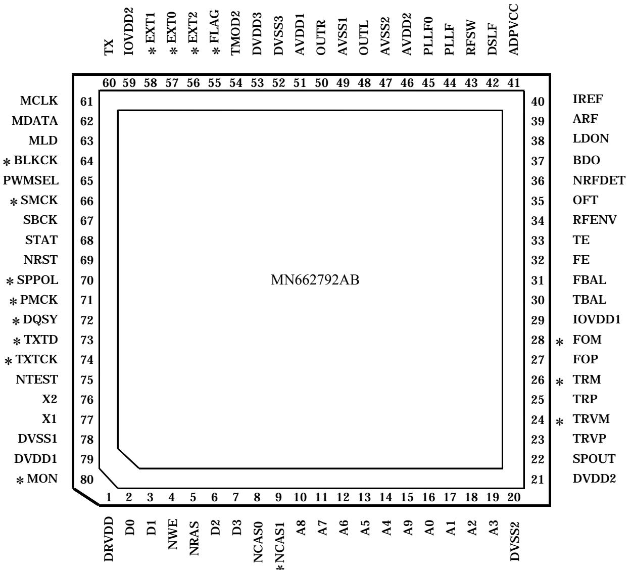
Note) Pins marked with an asterisk can be switched to different signals by using microcontroller commands.
