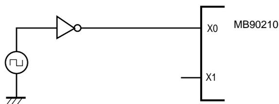
Note: When using an external clock, be sure to input external clock more than 6 machine cycles after setting the HST pin to "L" to transfer to the hardware standby mode.
