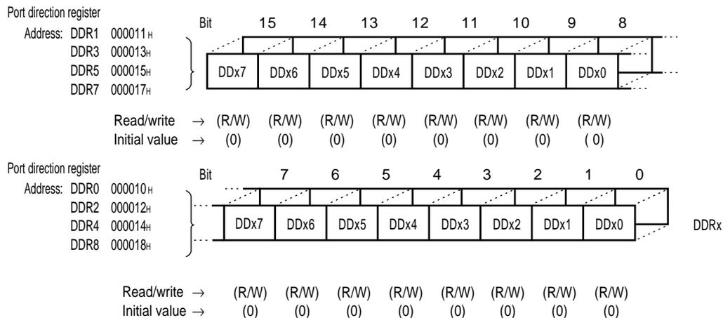
Note: No register bit is included in bits 7 and 6 of port 7 or bits 7 to 3 of port 8.
