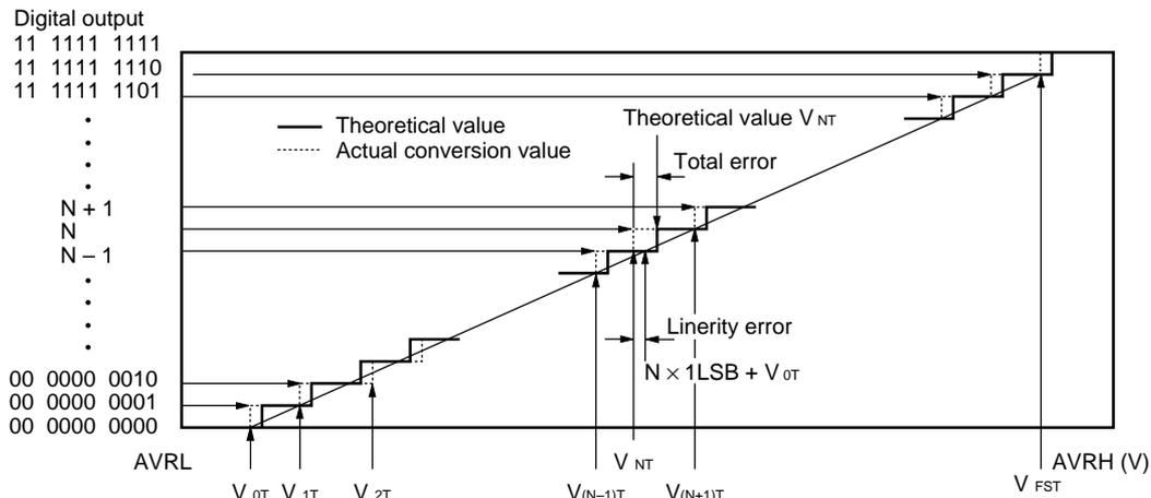
$$\bullet \text{ 1LSB} = \frac{V_{FST} - V_{OT}}{1022} \cdot \text{1LSB theoretical value} = \frac{AV_{RH} - AV_{RL}}{1022}$$
